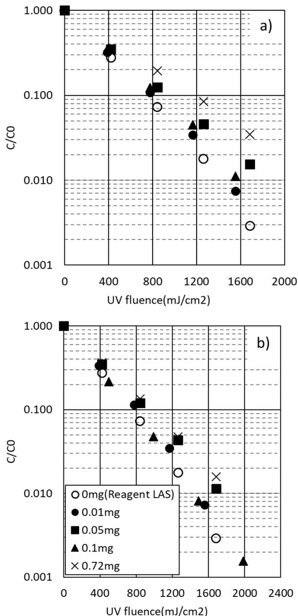
Fig. 4. Degradation effect of linear alkylbenzene sulfonate according to FWA concentration (a) FWA-1 and (b) FWA-5 (initial linear alkylbenzene sulfonate concentration: 12 mg/L).
