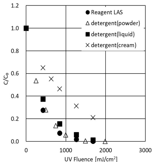
Fig. 2. Degradation of linear alkylbenzene sulfonate in different form (initial linear alkylbenzene sulfonate concentration: 12 mg/L).
