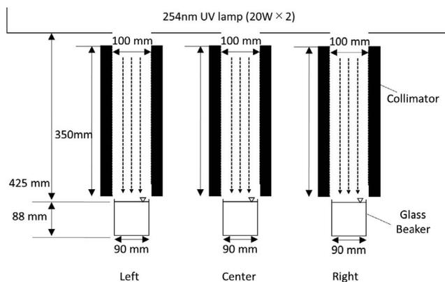
Fig. 1. Experimental set-up of a UV reactor.
