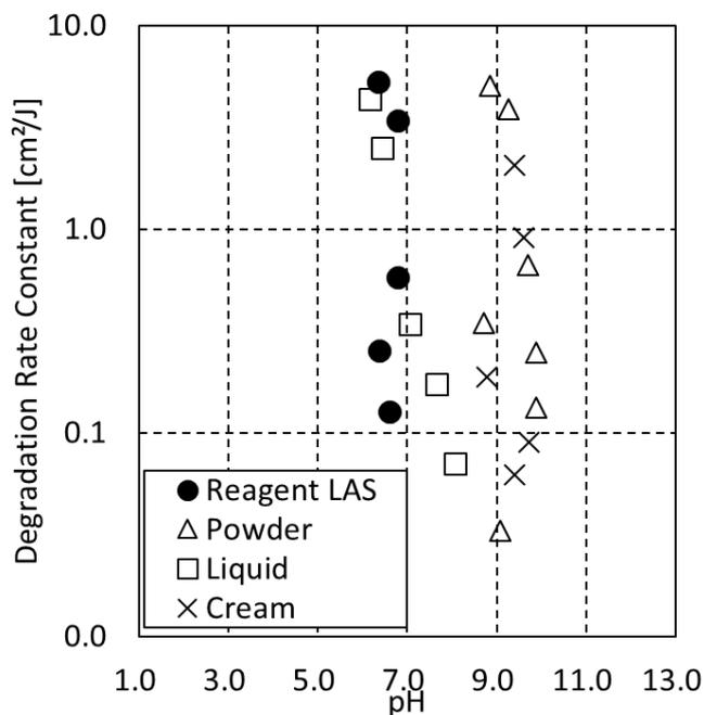
Fig. 3. Effect of pH on degradation of linear alkylbenzene sulfonate in a different form.
