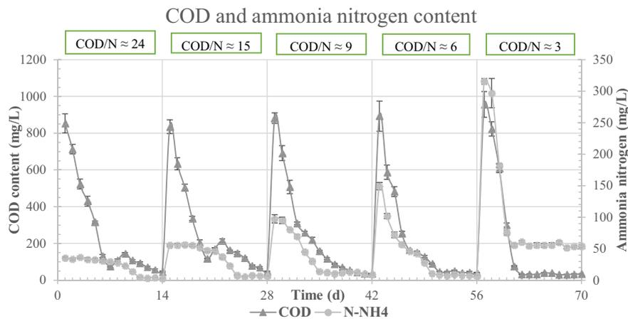
Fig. 2. Chemical oxygen demand and  $\text{N-NH}_4^+$  content during different cycles.
