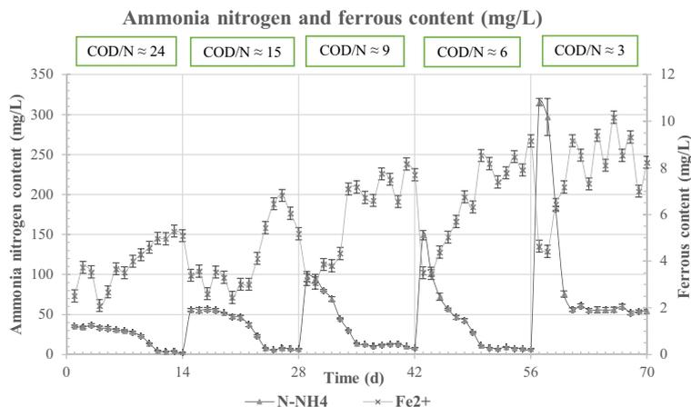
Fig. 3.  $\text{Fe}^{2+}$  and  $\text{N-NH}_4^+$  content during different cycles.
