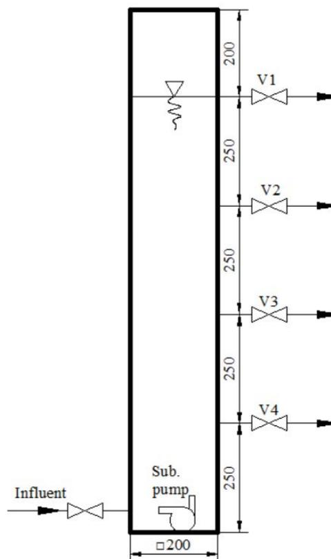
Fig. 1. Schematic diagram of the reactor.
