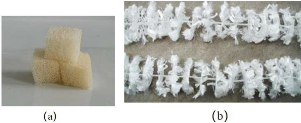
Fig. S1. Different fillers fed into the MBR system: (a) floating sponge filler and (b) combination filler.
