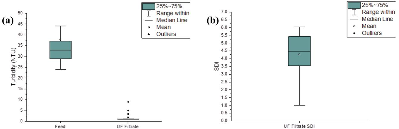
Fig. 7. (a) Feed and UF filtrate turbidity and (b) UF filtrate SDI.
