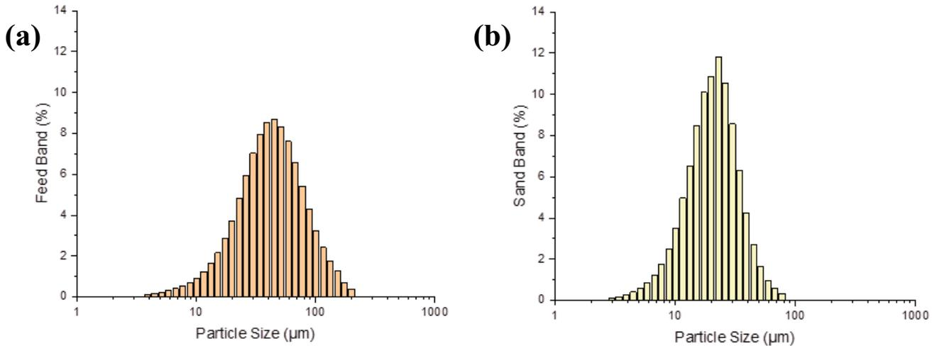
Fig. 6. Feed and media filter filtrate stream particle-size distribution.
