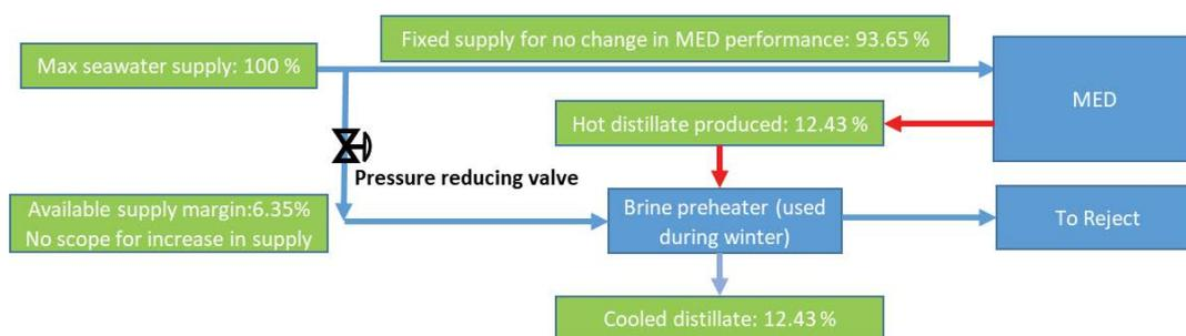
Fig. 5. Schematic representation showing the usage of available margin of seawater supply to reduce the distillate temperature in the preheater (brine cooler).
