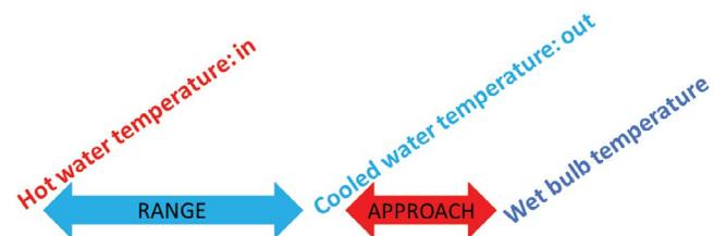
Fig. 1. Relationship between approach, range and wet-bulb temperature.
