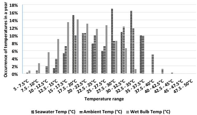
Fig. 3. Percent occurrence of different temperature ranges for the seawater, ambient temperature and the wet bulb temperature.
