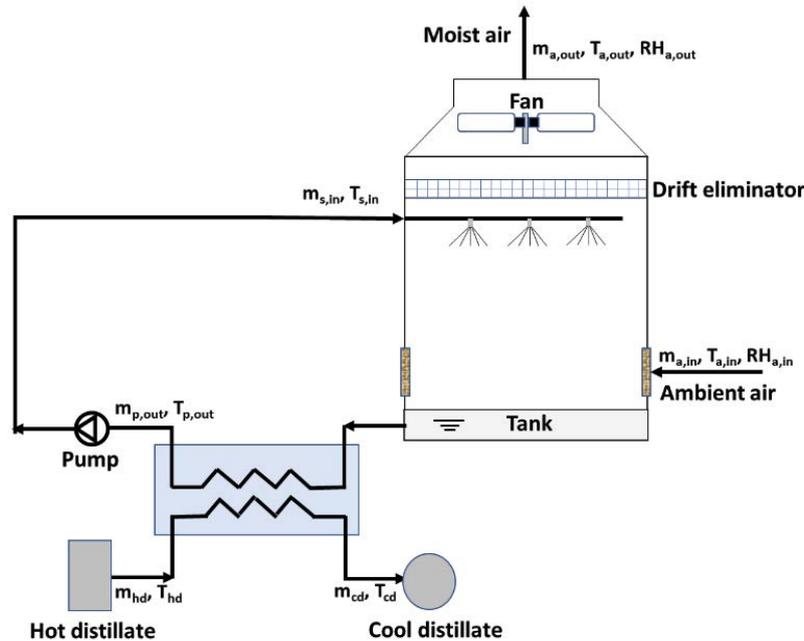
Fig. 8. Cooling tower with a heat exchanger used for cooling the hot distillate.
