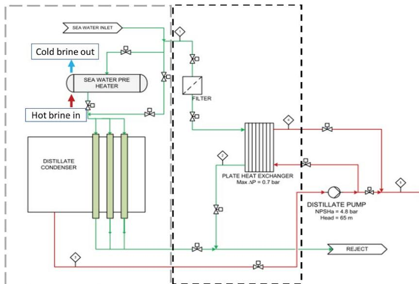
Fig. 4. Direct cooling of water (MED distillate) using seawater with plate type heat exchanger.
