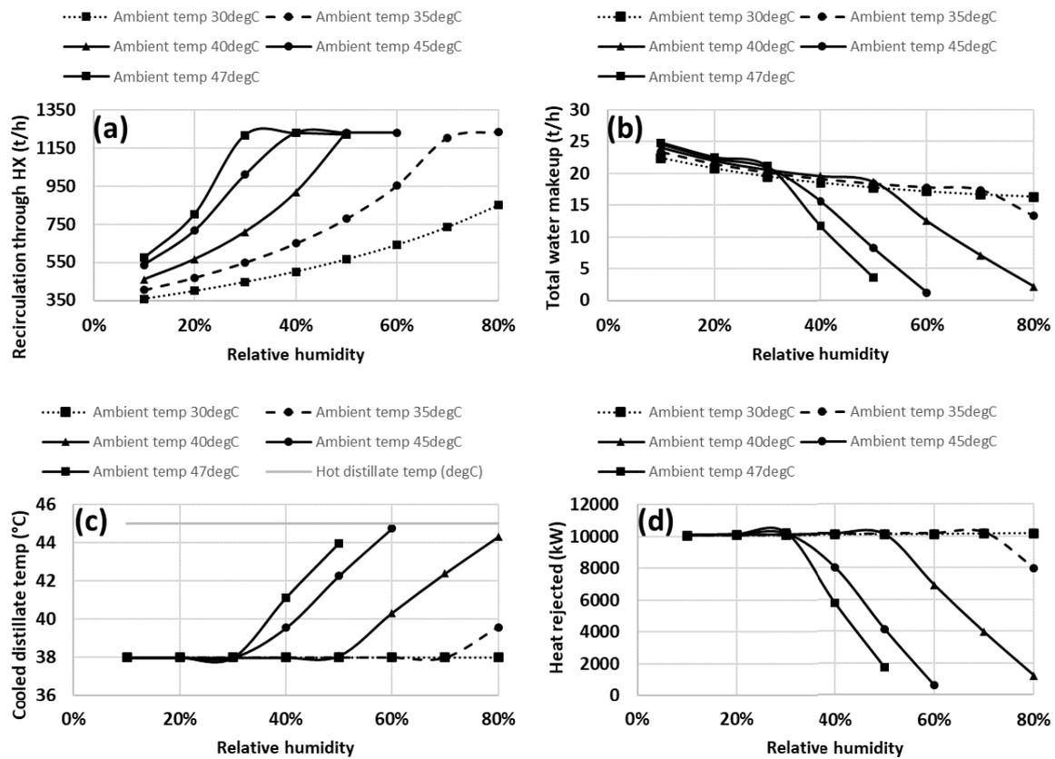
Fig. 10. (a) Variation of flow through the heat exchanger with relative humidity. (b) Variation of total water makeup with relative humidity. (c) Cooled distillate temperature achieved when the relative humidity is varied. Grey line represents the hot distillate temperature (45°C). (d) Heat rejected in the cooling tower when the relative humidity is varied.
