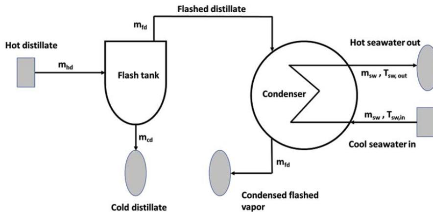
Fig. 6. Schematic representation showing the usage of available margin of seawater supply to reduce the distillate temperature in the preheater (brine cooler).
