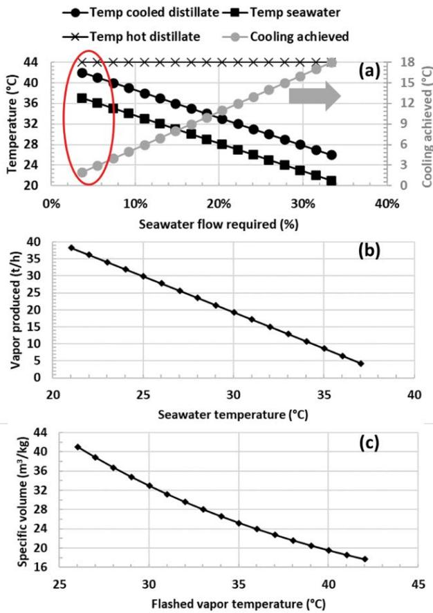
Fig. 7. (a) Temperature of seawater and cooled distillate at various seawater flows. Regimes covered under the available seawater flows are highlighted by the red ellipse. (b) Vapor produced in the flash vessel at various seawater temperatures. (c) Specific volume of the vapor produced in the flash vessel at various flashing temperatures.
