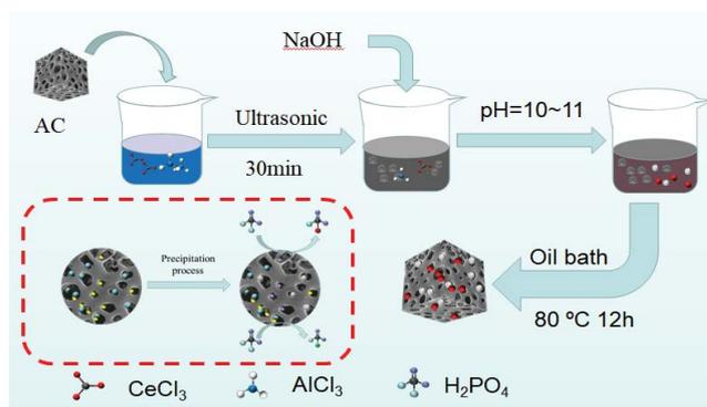
Fig. 2. Preparation of modified activated carbon and adsorption process.
