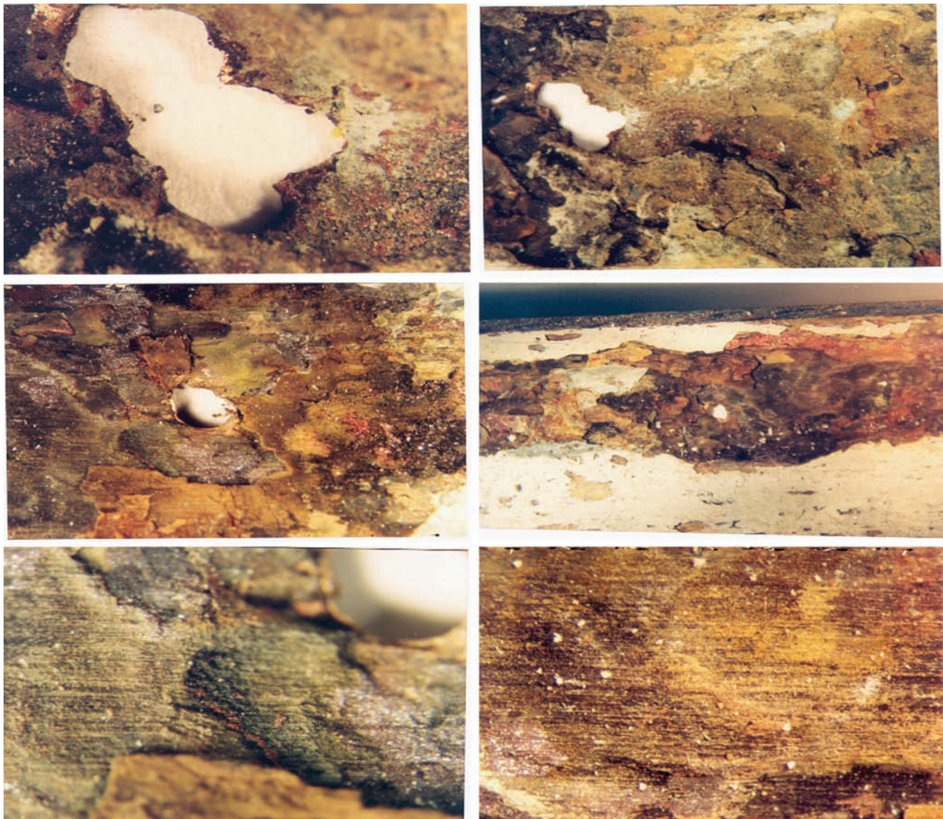
Fig. 3. Microscopic photograph of the inner part of the failed cupronickel condenser tubes (up to 40X).
