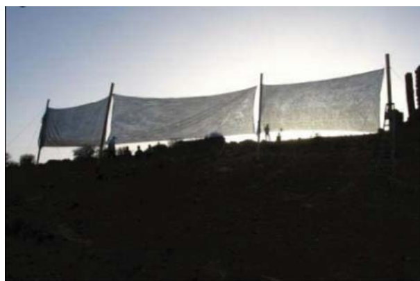
Fig. 5. Fog collector (F).
