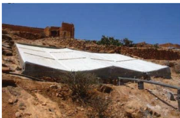
Fig. 4. Condenser on ground (CoG).
