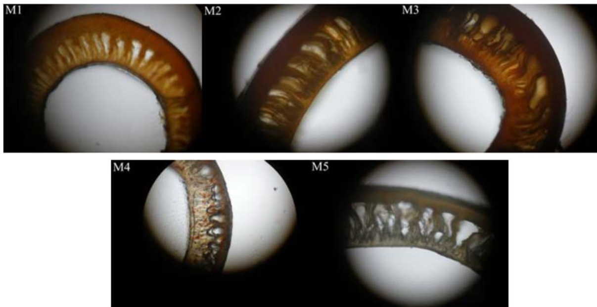
Fig. 1. PVDF/Fe 3+ /Cu 2+ hollow fiber membrane morphologies and Fe 3+ /Cu 2+ distributions in membranes under ordinary optical microscope.
