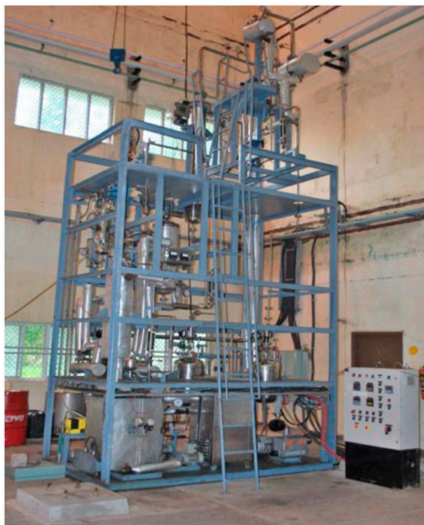
Fig. 1. Pilot plant solvent purification system.
