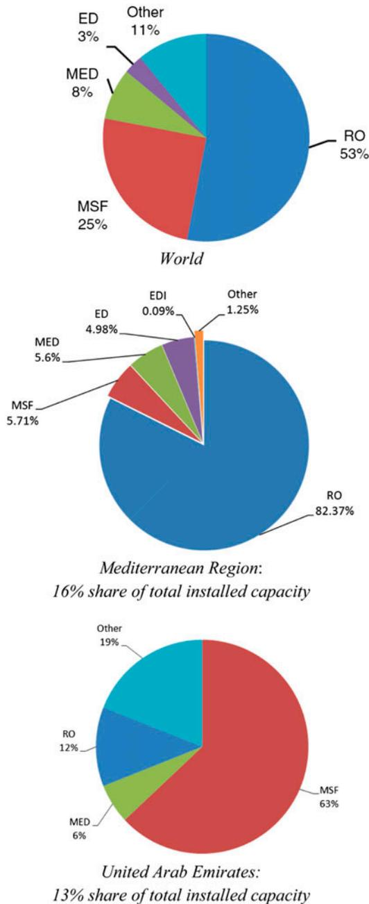
Fig. 1. Installed capacity by process, on a worldwide basis (top figure), the Mediterranean Sea (middle figure), and the United Arab Emirates (bottom figure). Notes: The data used for the graphics were taken from [2,4]. ED stands for Electrodialysis, EDI stands for Electro-dialysi Inversal.
