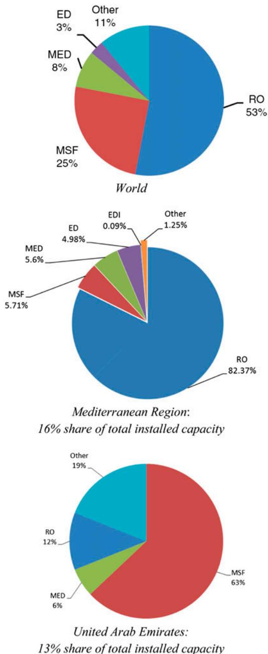
Fig. 1. Installed capacity by process, on a worldwide basis (top figure), the Mediterranean Sea (middle figure), and the United Arab Emirates (bottom figure).
