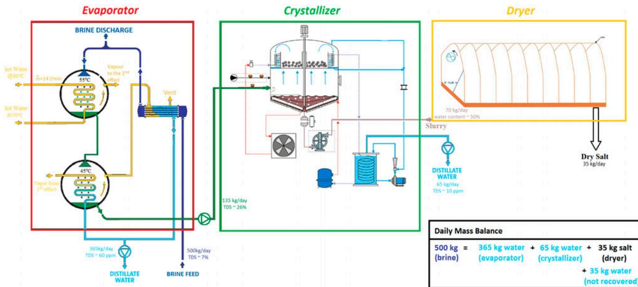
Fig. 6. Process flow diagram of the SOL-BRINE system. Note: The figures represent the daily mass balance of the system.
