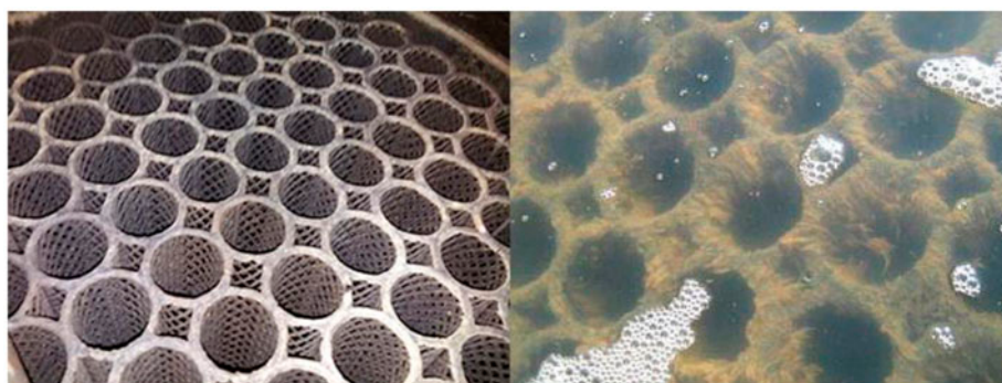
Fig. 2. Bio-filter in aerobic zones.
