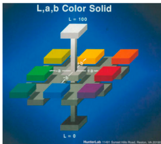
Fig. 1. Colour plotting diagram for L^* , a^* and b^* .
