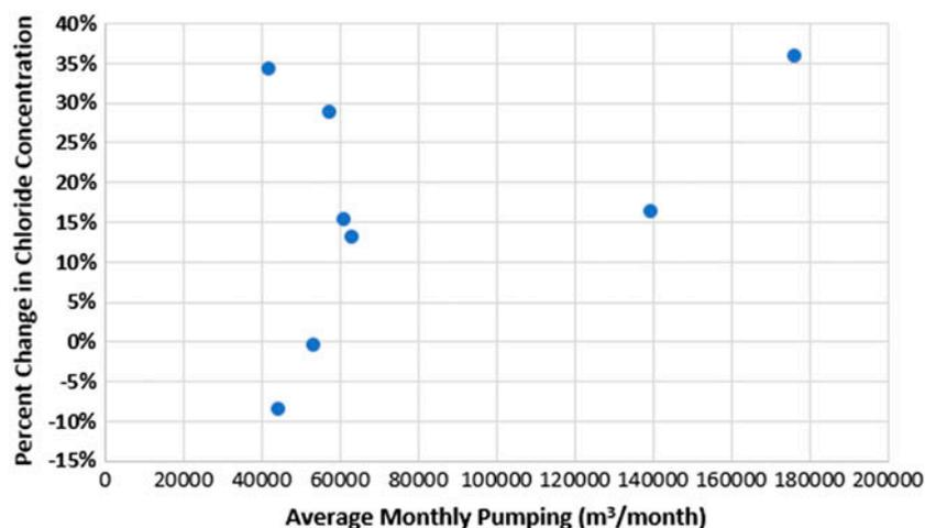
Fig. 5. Plot of average pumping rate per month vs. percentage change in dissolved chloride change.
