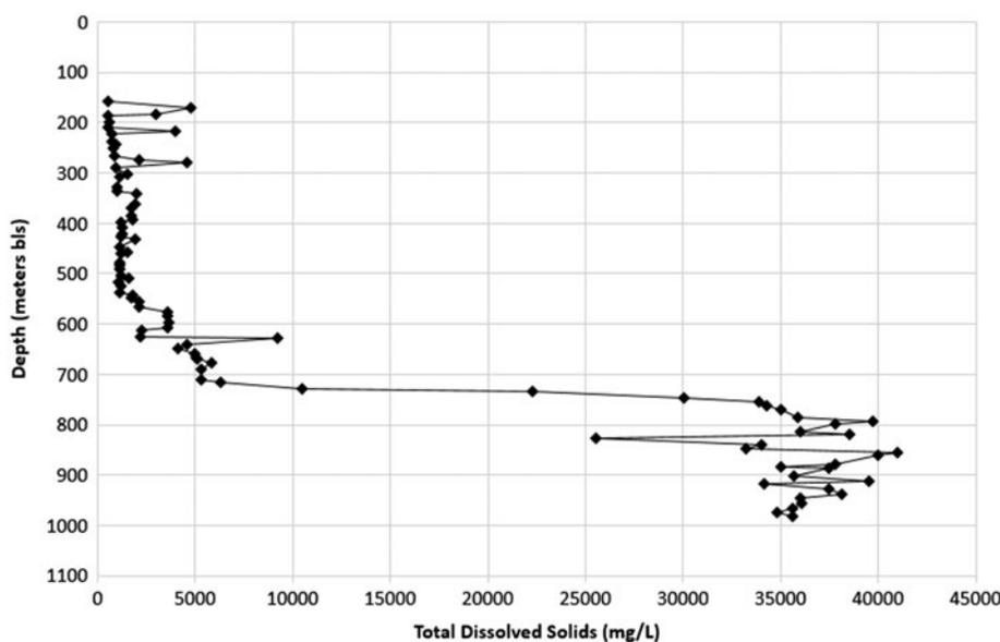
Fig. 3. Water quality variation with depth at the injection well test site.
