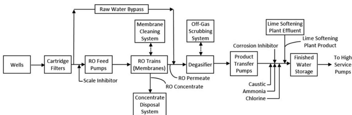
Fig. 7. Treatment process diagram for the Bonita Springs Utilities BWRO treatment plant.
