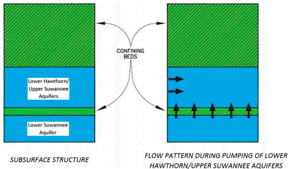
Fig. 6. Conceptual model used to assess projected future water quality changes within the production aquifer.
