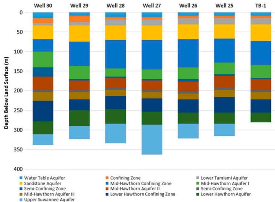
Fig. 2. Hydrogeologic cross-section of the Bonita Springs Utilities wellfield.
