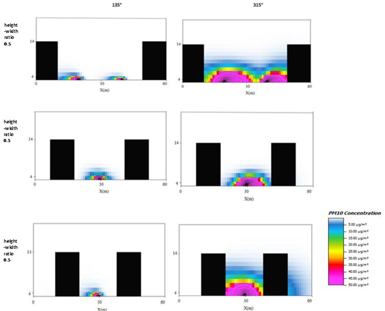
Fig. 4. Particle concentrations in the calm wind simulation (1 m/s) with different inflow directions (distance between contour lines is  $0.5 \mu\text{g}/\text{m}^3$ ).
