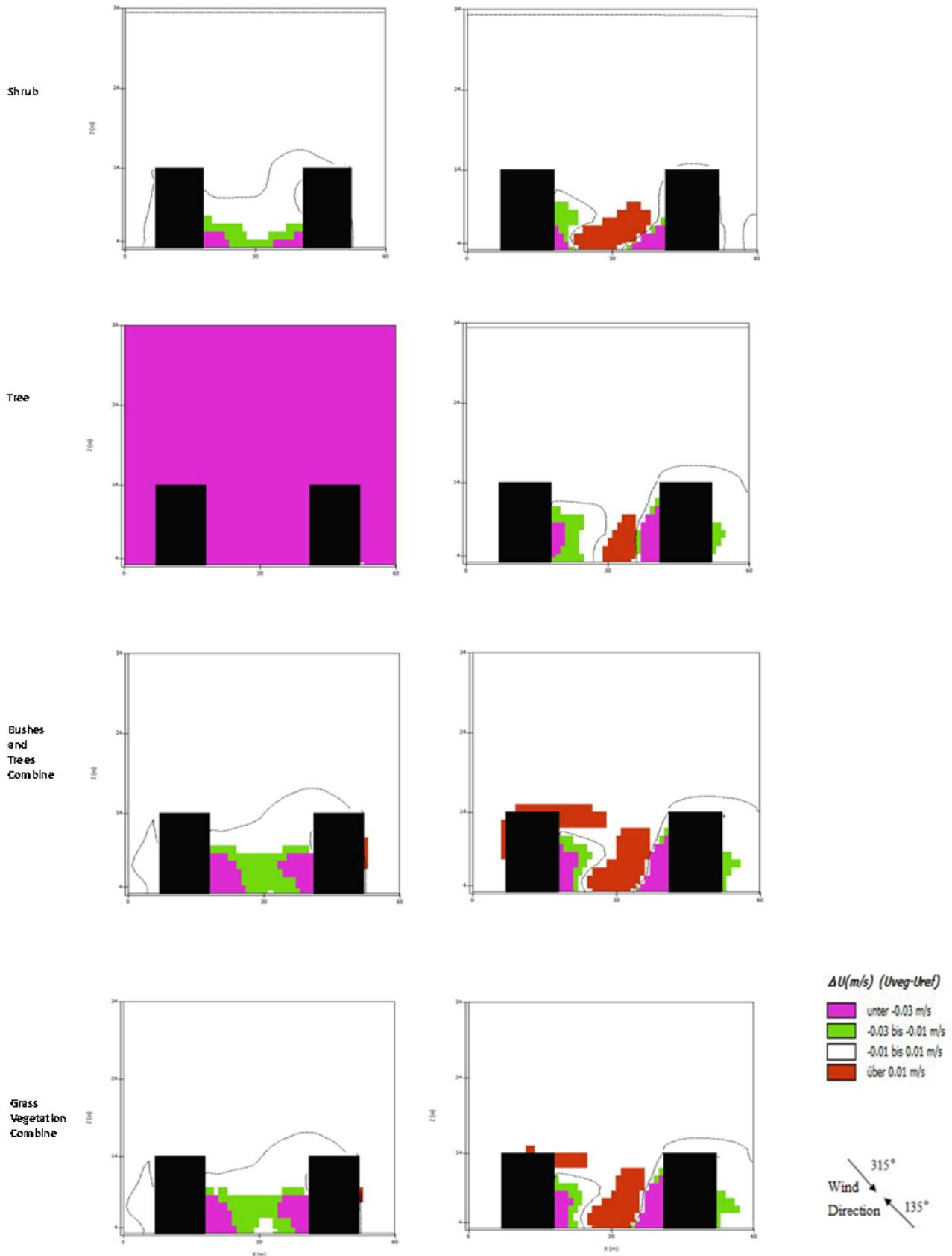
Fig. 6. Influence of vegetation on wind speed in the canyon with aspect ratio is 0.9 for the simulation with wind speed 1 m/s (reference case,  $U_{ref}$ ; vegetation scenarios,  $U_{veg}$ ).
