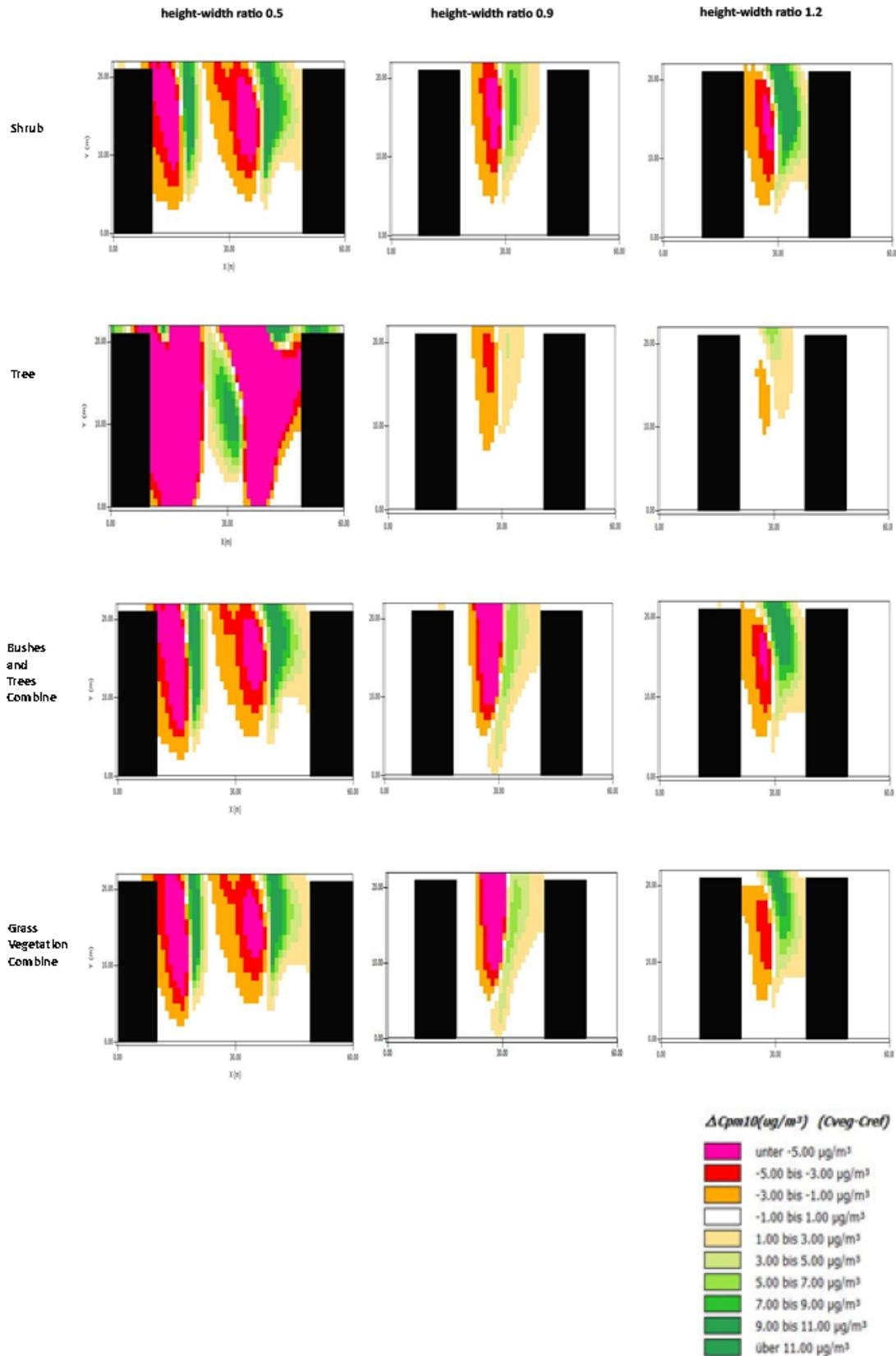
Fig. 5. Influence of vegetation on particle concentrations for inflow direction is 135° and wind speed is 1 m/s (grid cells at 1.5 m height). Comparison between the simulations without vegetation (reference case, Cref), with the hedge and the three tree scenarios (vegetation scenarios, Cveg).
