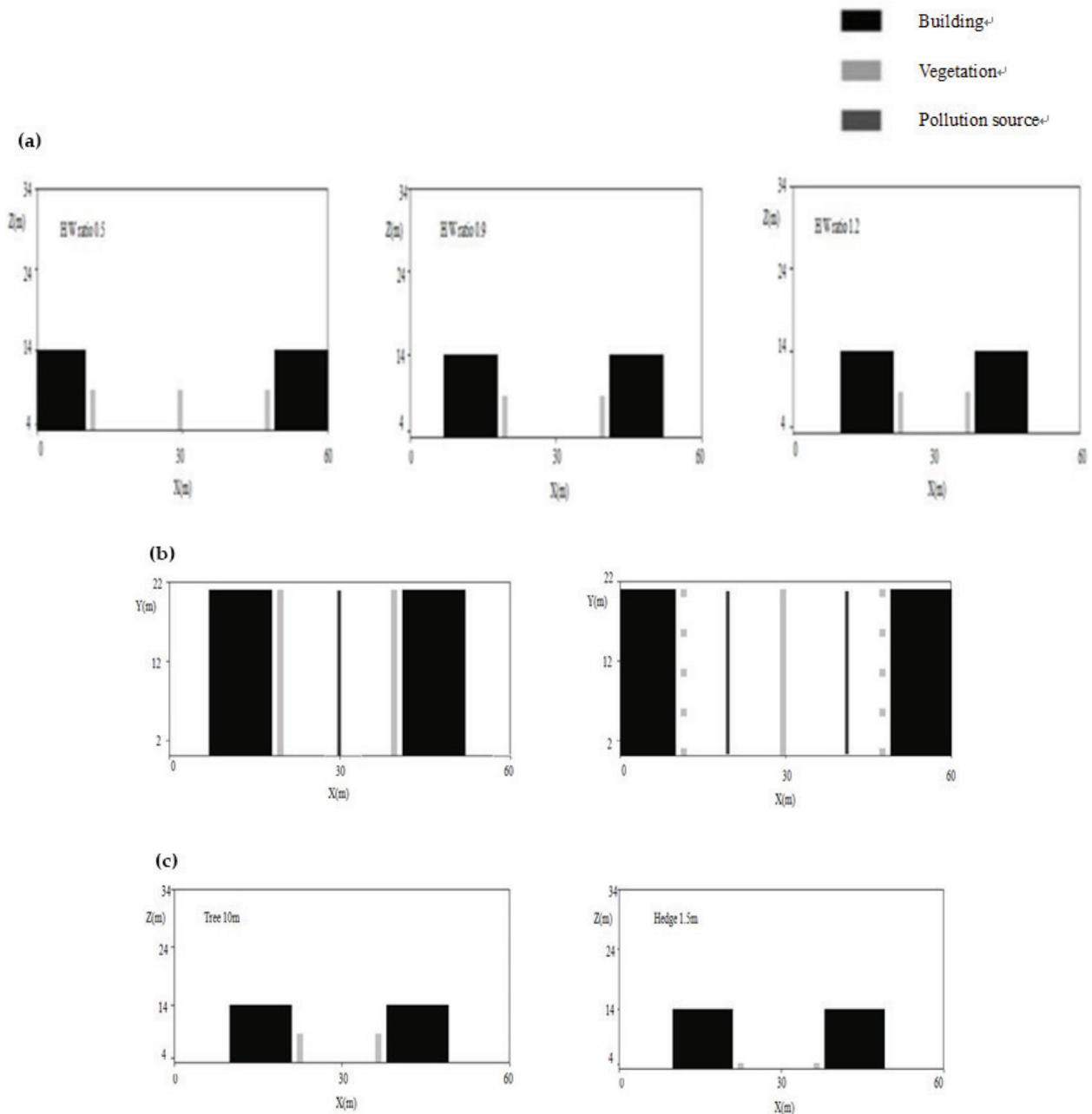
Fig. 2. (a) Cross section of all three aspect ratios, (b) plan view of model areas with (left) scenario with the widely spaced row of trees in the canyon with aspect ratio 0.9 and (right) scenario with continuous row of trees/hedge in the canyon with aspect ratio 0.5, and (c) a detailed view of the cross section with aspect ratio 0.9.
