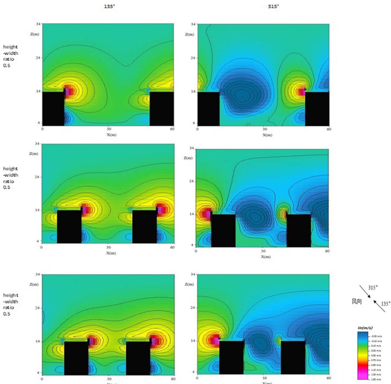
Fig. 3. Vertical wind flow ( $U_z$ ) with a wind speed at 10 m of 3 m/s. Blue colors indicate downward flow, green to magenta indicate upward flow (distance between contour lines is 0.1).
