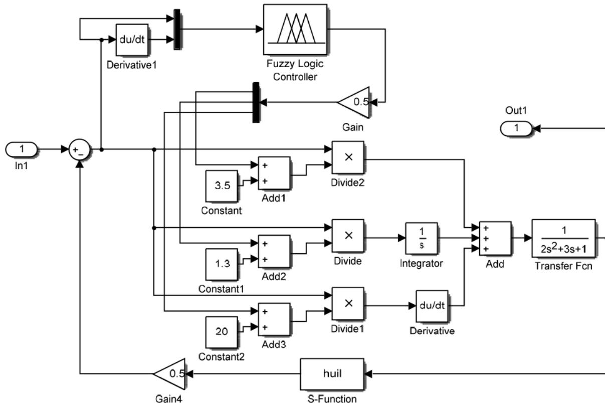
Fig. 8. Diagram of Simulink simulation.
