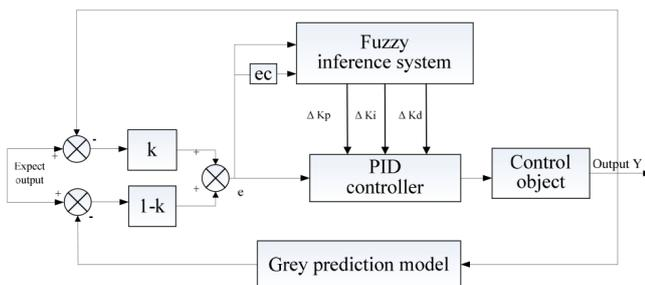
Fig. 7. Structure of grey prediction fuzzy-PID control for irrigation.
