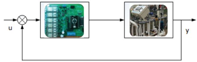
Fig. 1. Schematic diagram of water–fertilizer precision control.
