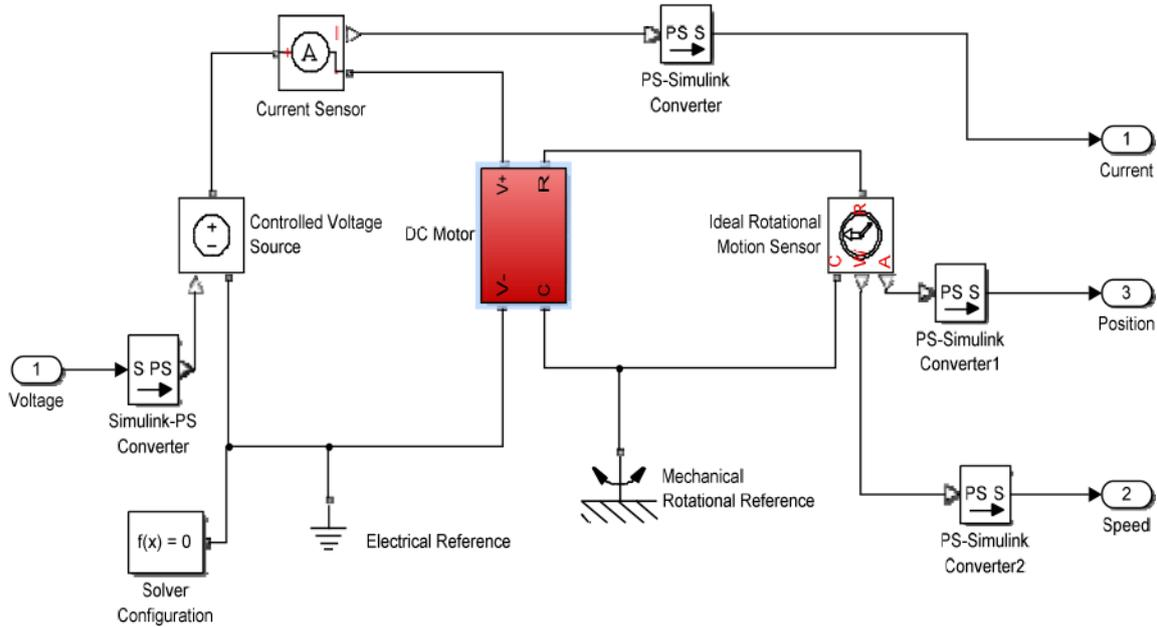
Fig. 5. Simulation model of DC motor Simscape.
