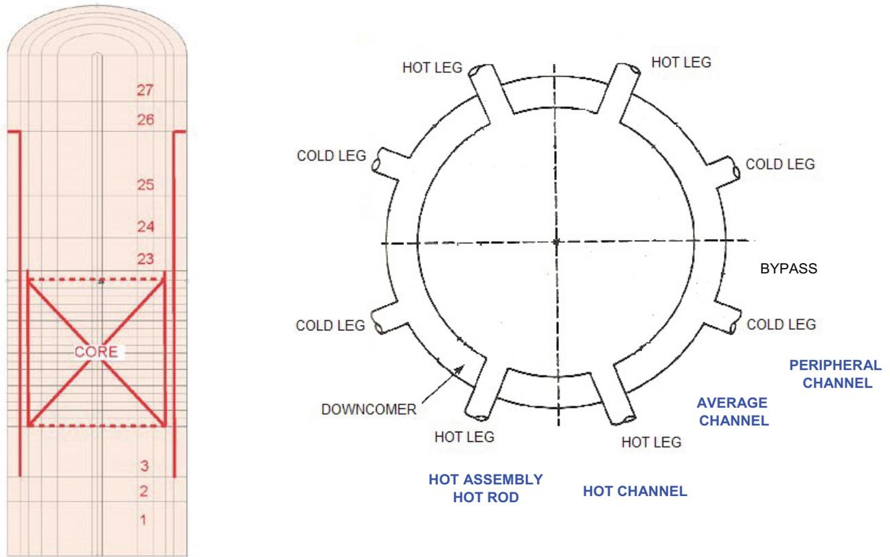
Fig. 2. 3-D nodalization for RPV.
