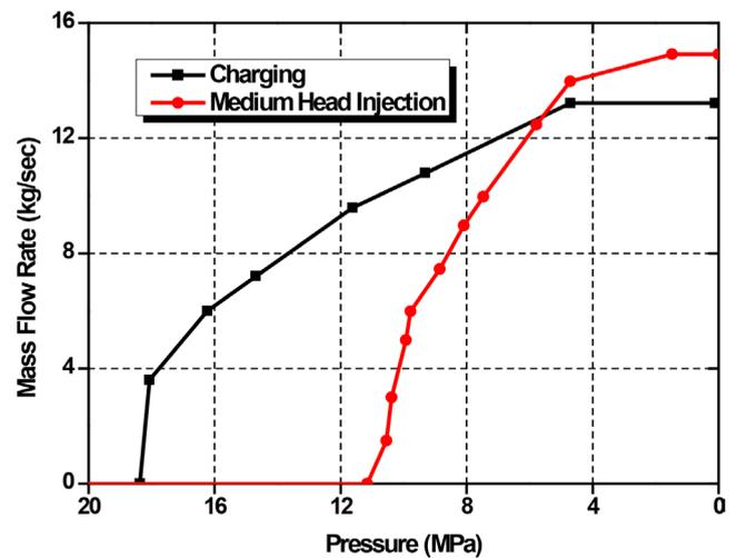
Fig. 3. Characteristics of charging and medium-head injection pumps.
