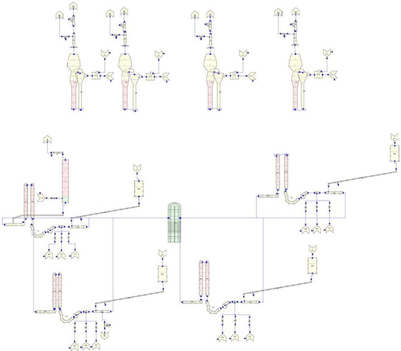
Fig. 1. Nodalization of Zion nuclear power plant.
