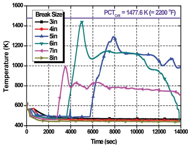
Fig. 4. Time trace of maximum PCT (with HPI).
