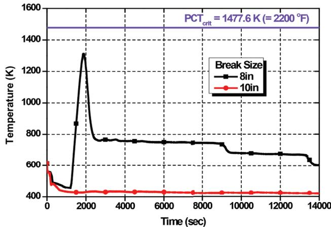
Fig. 8. Comparison of maximum PCTs between 8 and 10 in breaks.
