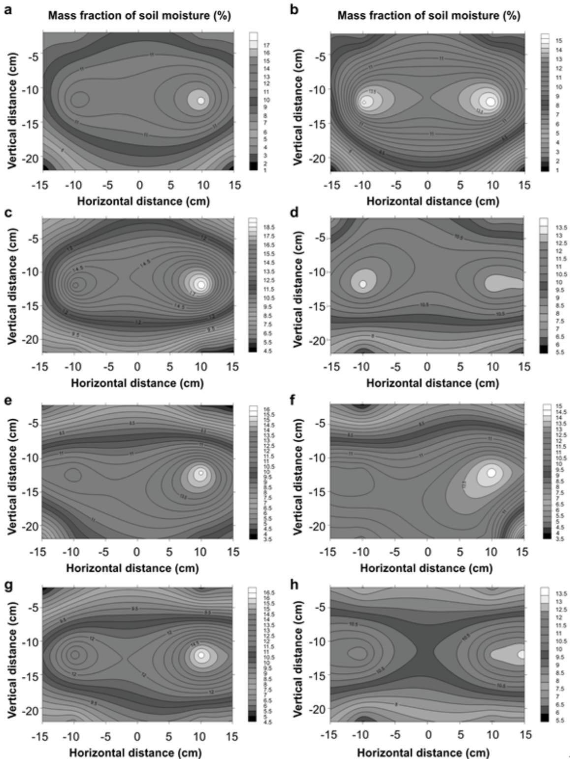
Fig. 3. Water distribution in two soils in two emitter modes under root infiltration irrigation: (a)  $x$ -axis profile of IGDTSR, (b)  $y$ -axis profiles of IGDTSR, (c)  $x$ -axis profile of IGSSR, (d)  $y$ -axis profiles of IGSSR, (e)  $x$ -axis profile of IGDTSY, (f)  $y$ -axis profiles of IGDTSY, (g)  $x$ -axis profile of IGSSY, (h)  $y$ -axis profiles of IGSSY.
