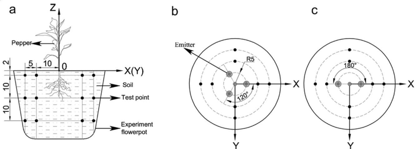
Fig. 2. Schematic diagram of soil moisture content measurement arrangement: (a) distribution of measuring points on the x(y)-axis profile; (b) top view of emitter in DT mode; (c) top view of emitter in DS mode.
