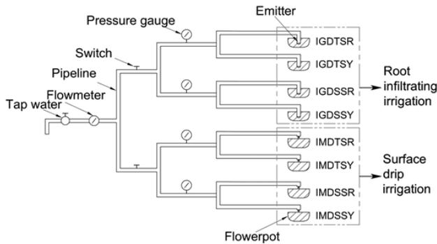
Fig. 1. Sketch of the test system used in the experiments.
