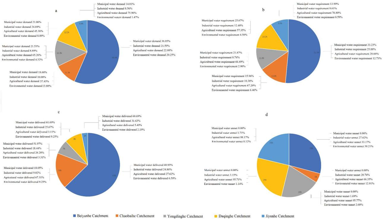
Fig. 8. Water demand computed by Beijing WEAP 2010 in different catchments: a – water demand; b – supply requirement; c – supply delivered; d – unmet demand.
