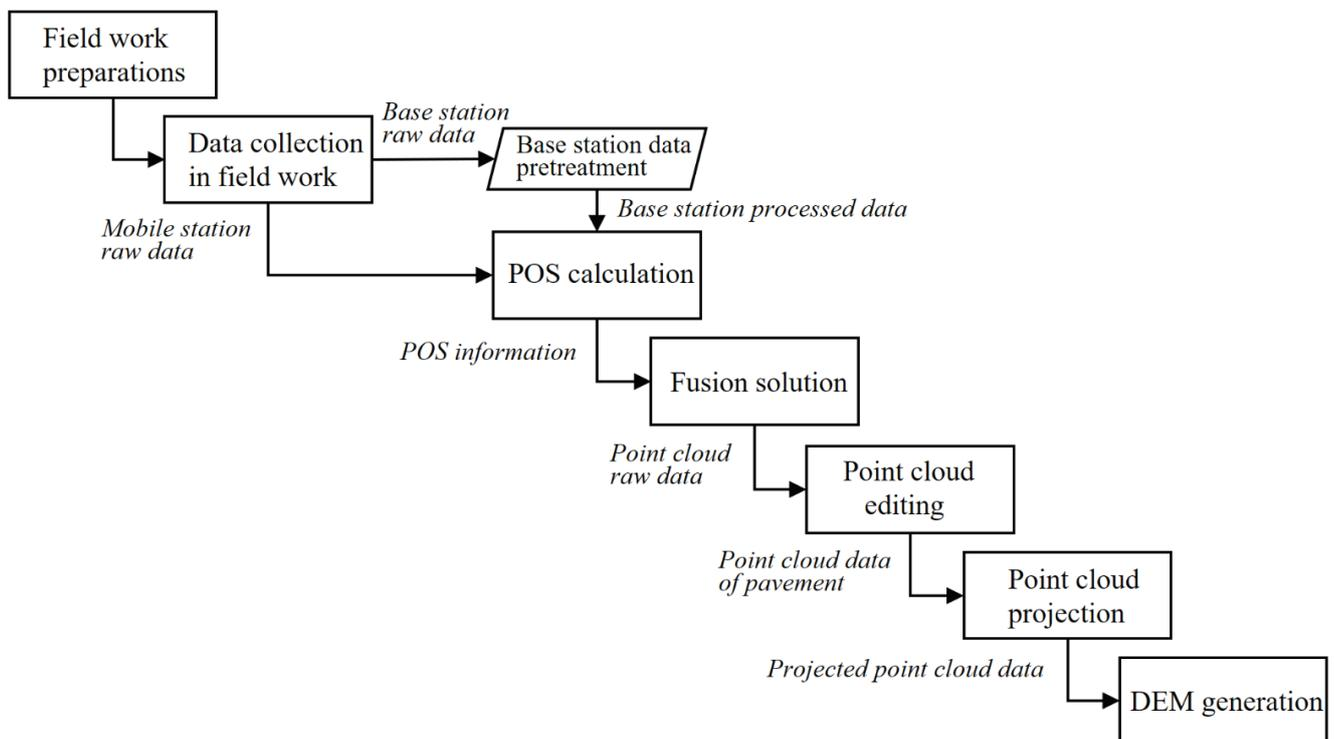
Fig. 1. Processes of DEM construction from LiDAR for land vehicles.
