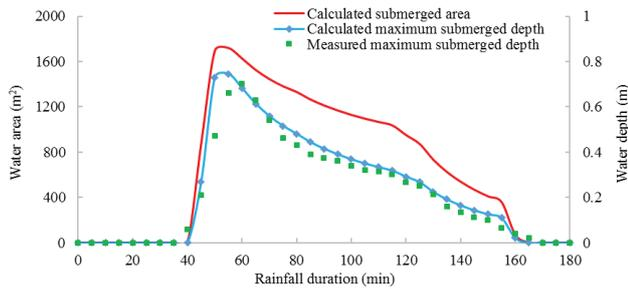
Fig. 10. Comparison between the calculated results and the measured results of submerged information.
