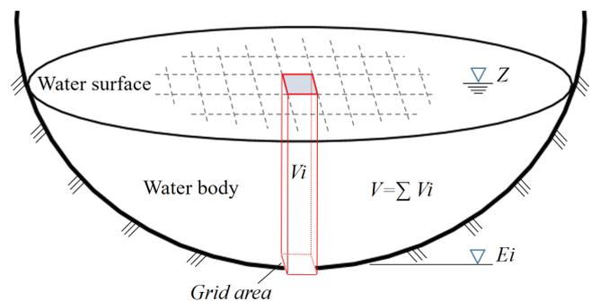
Fig. 3. Diagram of the calculation of water accumulation volume in inundate area.
