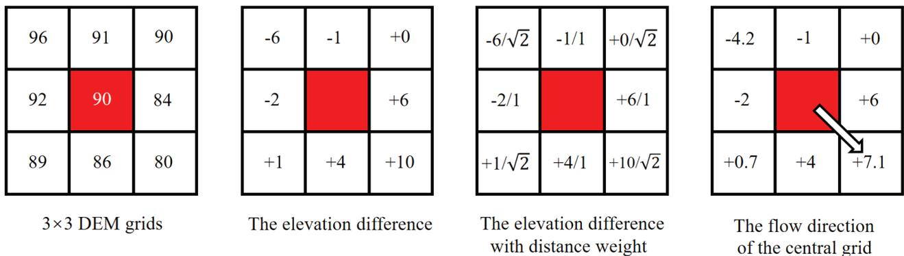
Fig. 2. The process of the D8 algorithm.
