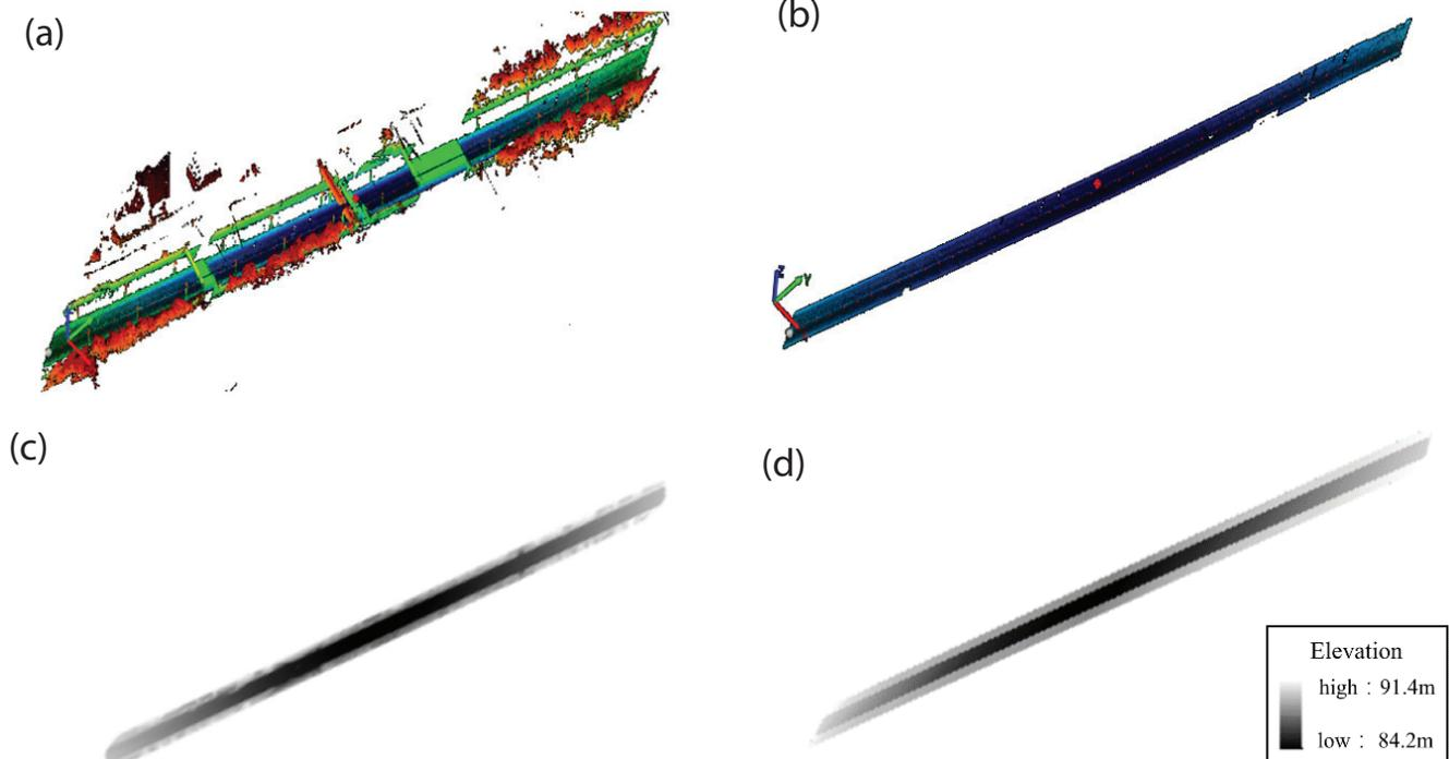
Fig. 5. Generation process of the DEM data in the studied inundate area: (a) point cloud raw data, (b) point cloud edited data of pavement, (c) generated DEM data after projection, and (d) DEM edited data.
