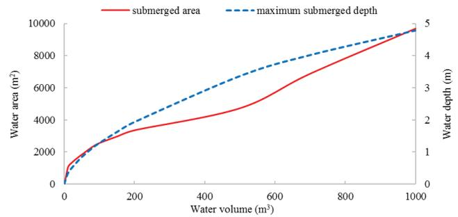
Fig. 8. The relation curves of water volume and submerged features of the studied inundate area.
