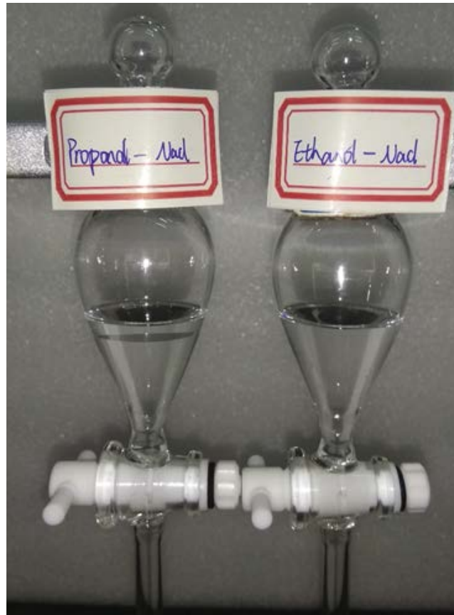
Fig. S2. The photo of the stratification of the n -propanol-NaCl and the ethanol-NaCl systems ( \Pi_0 50 \mu\text{mol/L} , 1.6 g NaCl, 6 mL wastewater, 3 mL alcohols, 1 mL HCl (1 mol/L), 3 min contact time, and 298 K).
