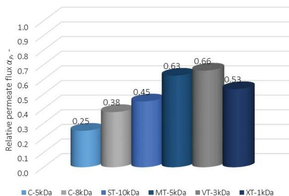
Fig. 8. Relative permeate fluxes through polymeric and ceramic membranes applied in treatment of biological effluents (TMP of 0.3 MPa).
