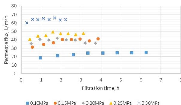
Fig. 4. Permeate flux for MT-5 kDa membrane as a function of transmembrane pressure in the range of 0.1–0.3 MPa.
