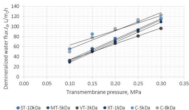
Fig. 2. Deionized water flux determined for tested PES and ceramic membranes as a function of transmembrane pressure in the range of 0.1–0.3 MPa.
