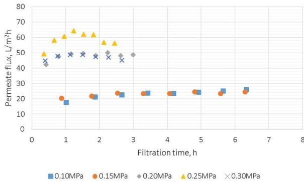
Fig. 5. Permeate flux for VT-3 kDa membrane as a function of transmembrane pressure in the range of 0.1–0.3 MPa.
