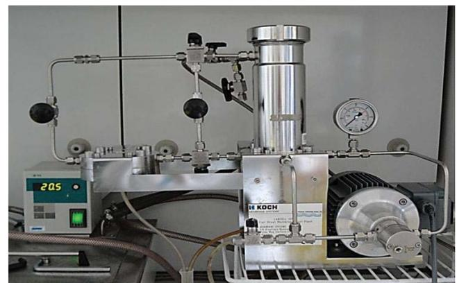
Fig. 1. KMS Cell CF1 laboratory-scale membrane filtration unit.
