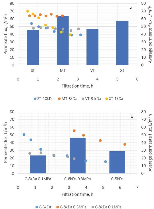
Fig. 7. The change of permeate flux with filtration time and its average value for biological effluent ultrafiltration (TMP of 0.3 MPa) for tested PES (a) and ceramic (b) membranes.
