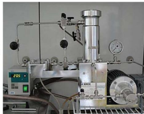
Fig. 3. KMS Cell CF1 laboratory-scale membrane filtration unit.
