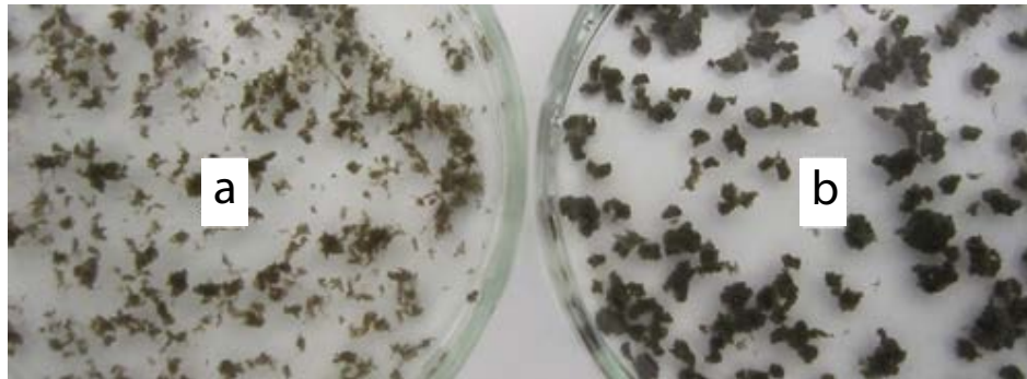
Fig. 7. Images of sludge conditioned by single CPAM (a) and dual conditioners (b).
