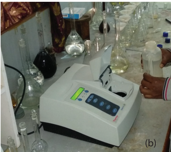
Fig. 7. (a) Water sample collection at Node J6 (23°49'17.61"N, 86°27'35.25"E) is shown. (b) Laboratory test of the water samples collected in Path-I for finding out residual chlorine concentration.
