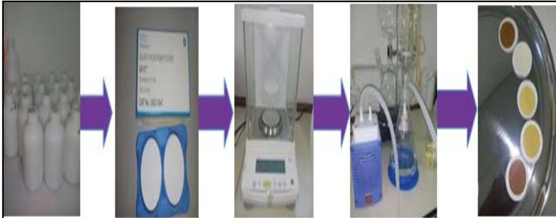
Fig. 6. Gravimetric method to analyse the total suspended solid (TSS).
