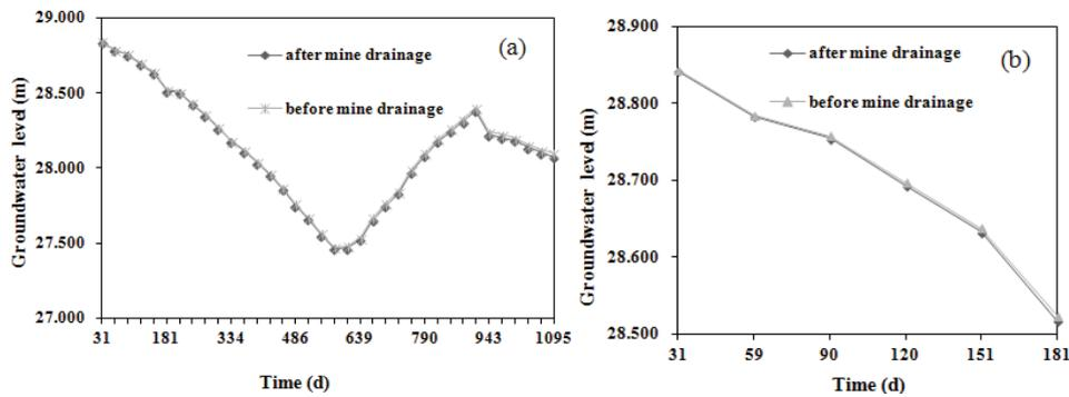
Fig. 4. The hydrograph of water level before and after mine drainage. (a) The hydrograph in 1,095 d and (b) the hydrograph in 181 d.
