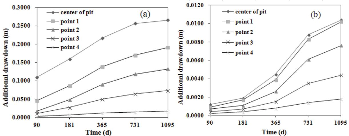
Fig. 6. The additional drawdown (a) hydrograph of karst water and (b) pore water without water bursting.
