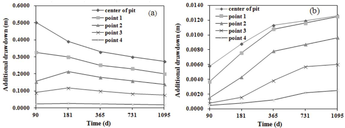
Fig. 5. The additional drawdown (a) hydrograph of karst water and (b) pore water with water bursting.
