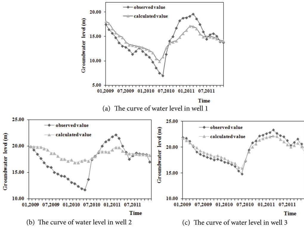
Fig. 3. The correlation curve of calculated water level and observed water level in observation wells 1, 2, and 3.
