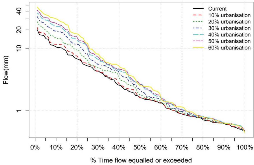
Fig. 7. Flow duration curve at different levels of impervious cover.
