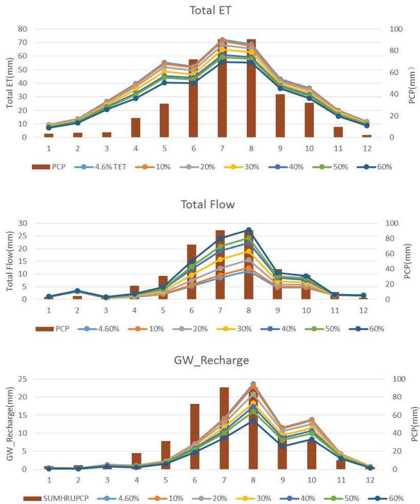
Fig. 8. Effect of impervious cover on total ET, total flow, and groundwater levels at average monthly scale.
