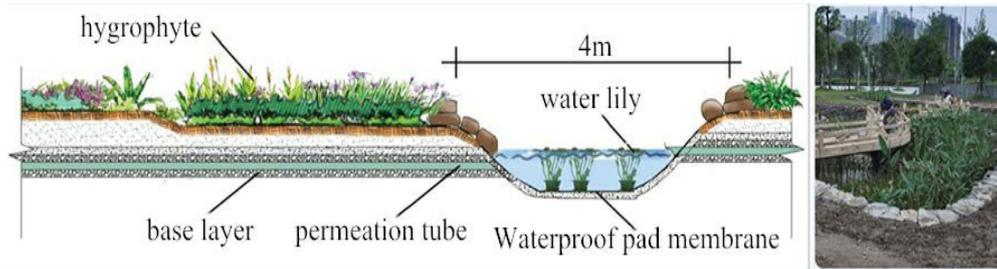
Fig. 2. Cross section and image of a bioretention pond (Source: <http://www.tidelion.com/hxpro/chengpin/>).
