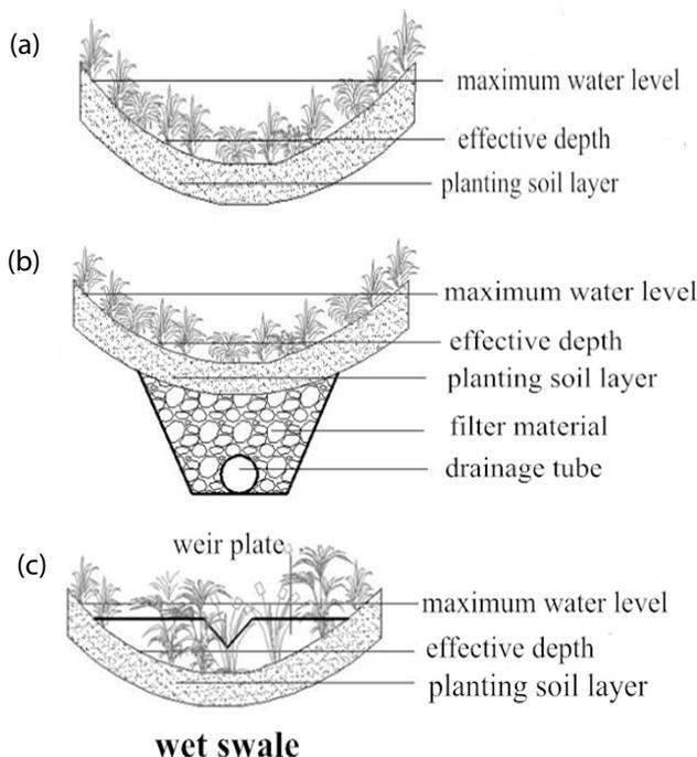
Fig. 1. (a) Cross section of a standard transmission swale, (b) cross section of a dry swale, and (c) cross section of a wet swale (cite from: *Research on the running effect evaluation and improvement design of grass swale. Dissertation*).
