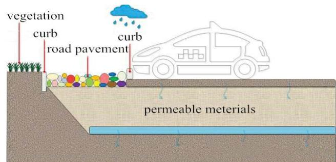
Fig. 3. Cross section of a permeable pavement installation (Source: <http://www.17wh.com/cjm/20170206/1509105.html>).
