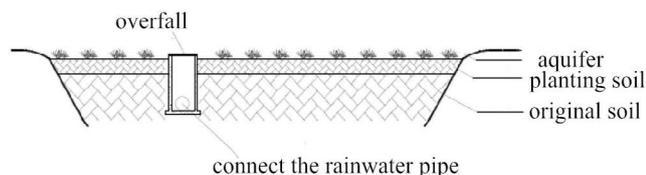
Fig. 4. Cross section of a low-elevation greenbelt (Source: [http://www.fwjia.com/2016/0402/411797\\_2.html](http://www.fwjia.com/2016/0402/411797_2.html)).
