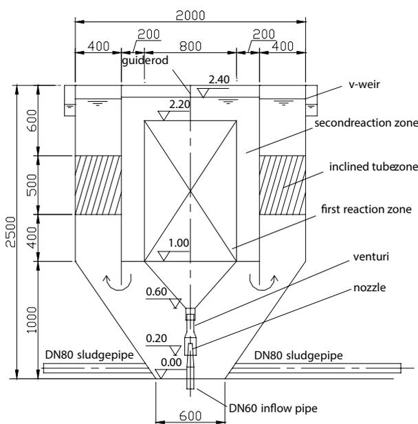
Fig. 1. Structure diagram of micro-vortex clarifier.
