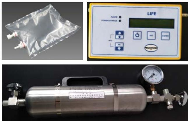
Fig. 2. Tedlar gas sample bags and gas sampler.
