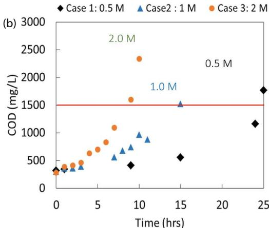
Fig. 4. Results of the FO process for wastewater concentration using different concentrations for the draw solution. (a) Concentration factor, (b) COD concentration levels.
