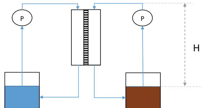
Fig. 3. Considered pumping arrangement for circulation energy requirement calculation.
