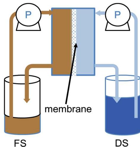
Fig. 1. Experimental layout.
