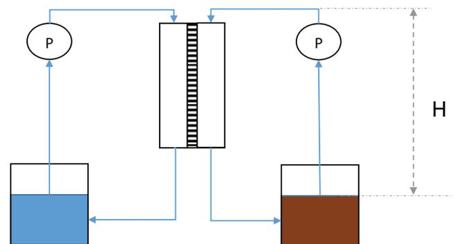
Fig. 3. Considered pumping arrangement for circulation energy requirement calculation.
