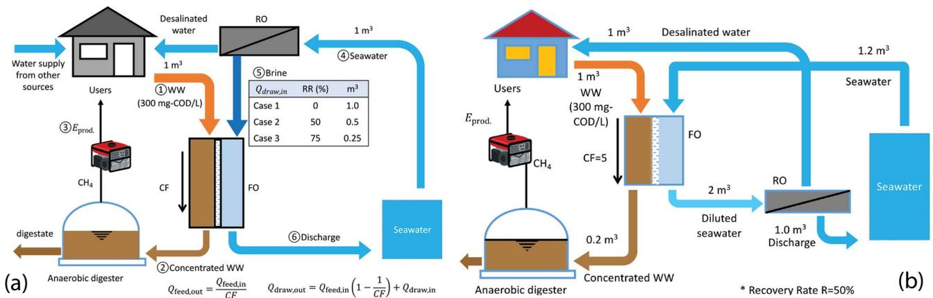
Fig. 2. Two different scenarios considered in this study: (a) FO following RO and (b) RO following FO.
