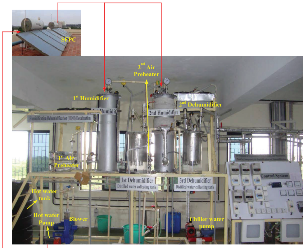
Fig. 1. Experimental setup of solar flat plate collectors assisted two stage humidification-dehumidification desalination and cooling plant.
