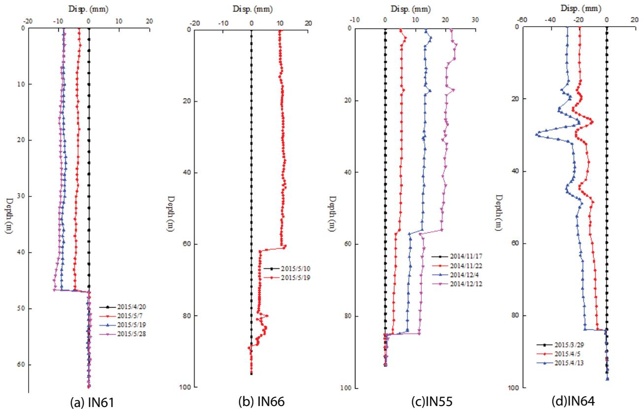
Fig. 4. Curves of displacement vs. depth indicated by inclinometer.
