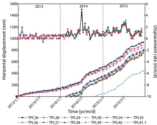
Fig. 6. Horizontal displacement vs. time, displacement rate vs. time curves of LMG during the monitoring period.
