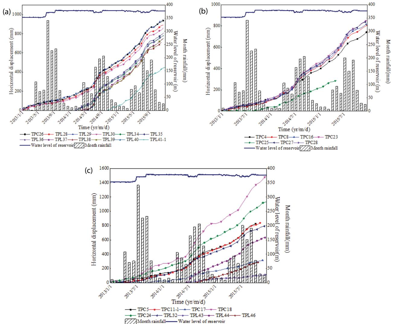
Fig. 10. Relationship between cumulative displacement, rainfall, and the reservoir water level (a) LMG, (b) CP1, and (c) GBP1.
