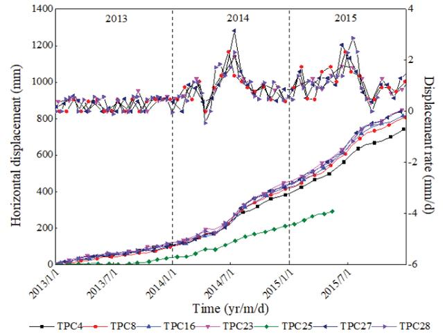
Fig. 7. Horizontal displacement vs. time, displacement rate vs. time curves of CP1 during the monitoring.
