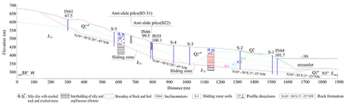
Fig. 3. Schematic geological cross-section (A-A') of the landslide.
