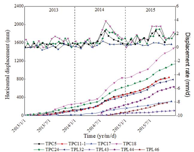
Fig. 8. Horizontal displacement vs. time, displacement rate vs. time curves of GBP1 during the monitoring period.
