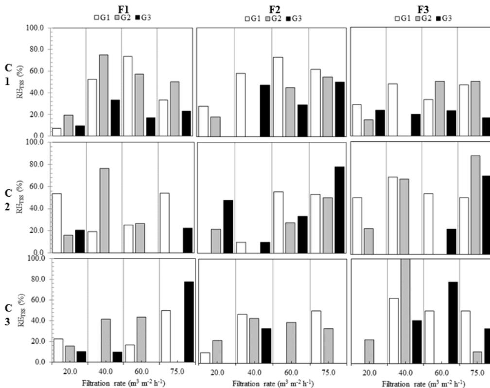
Fig. 6. Filtration removal efficiency using TSS from water samples ( $RE_{TSS}$ ) (%) considering the third sampling (240 min) for different sand particle size and filtration rate combinations for the filtration cycles C1, C2 and C3.
