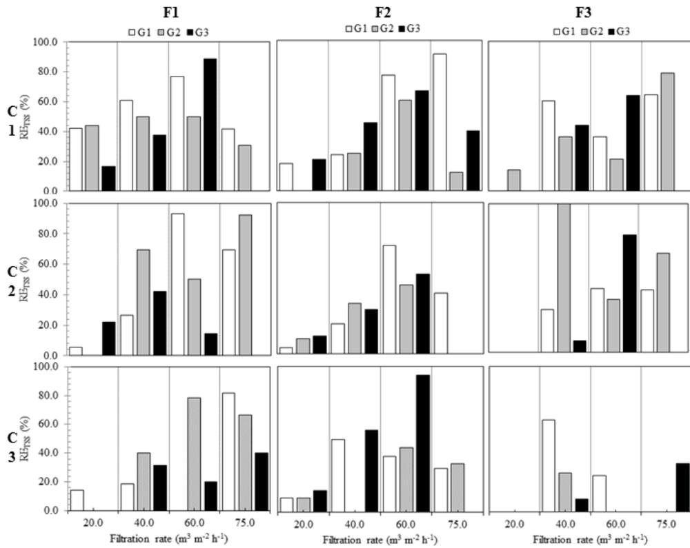
Fig. 5. Filtration removal efficiency using TSS from water samples ( $RE_{TSS}$ ) (%) considering the second sampling (120 min) for different sand particle size and filtration rate combinations for the filtration cycles C1, C2 and C3.
