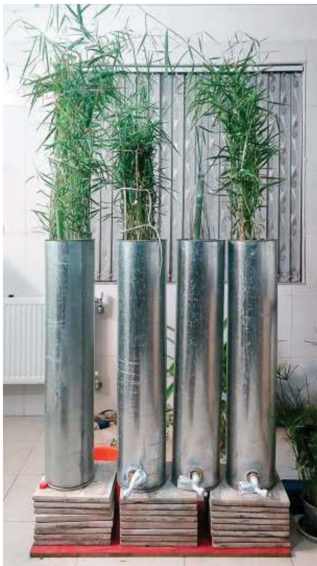
Fig. 4. Vertical flow constructed wetlands during the sampling, indoors with temperature range of 18°C–24°C.
