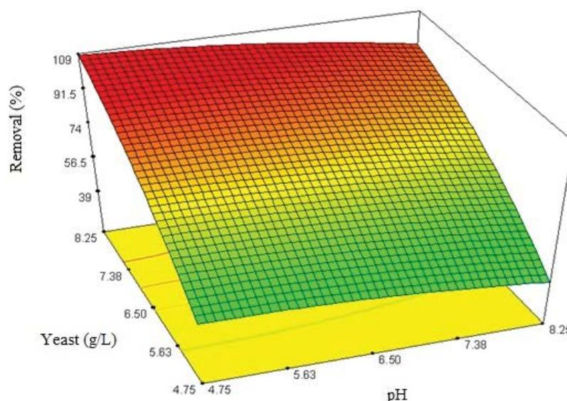
Fig. 5. Effect of pH and adsorbent dosage on the removal of RR 120 at the dye concentration of 27.5 mg L<sup>-1</sup> and the reaction time of 95 min.
