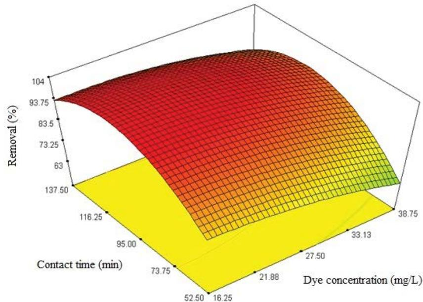
Fig. 4. Effect of contact time and initial color concentration on the removal of RR 120 at the pH of 6.5 and the yeast dose of 6.5 g L<sup>-1</sup>.
