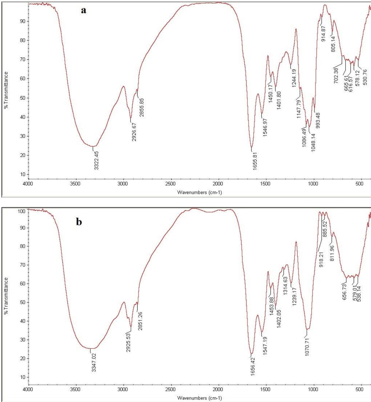
Fig. 2. FTIR analysis for *S. cerevisiae* (a) before and (b) after the adsorption of dye.
