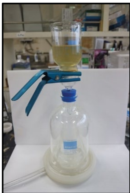
Fig. 2. Filtration of treated sewage effluent after collection.
