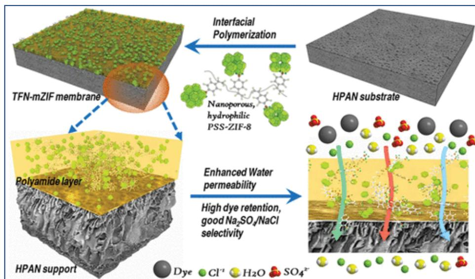
Fig. 1. Schematic of a TFN membrane containing poly (sodium 4 styrenesulfonate; PSS) modified ZIF-8 (mZIF) in a polyamide (PA) layer were constructed. Source, [17].
