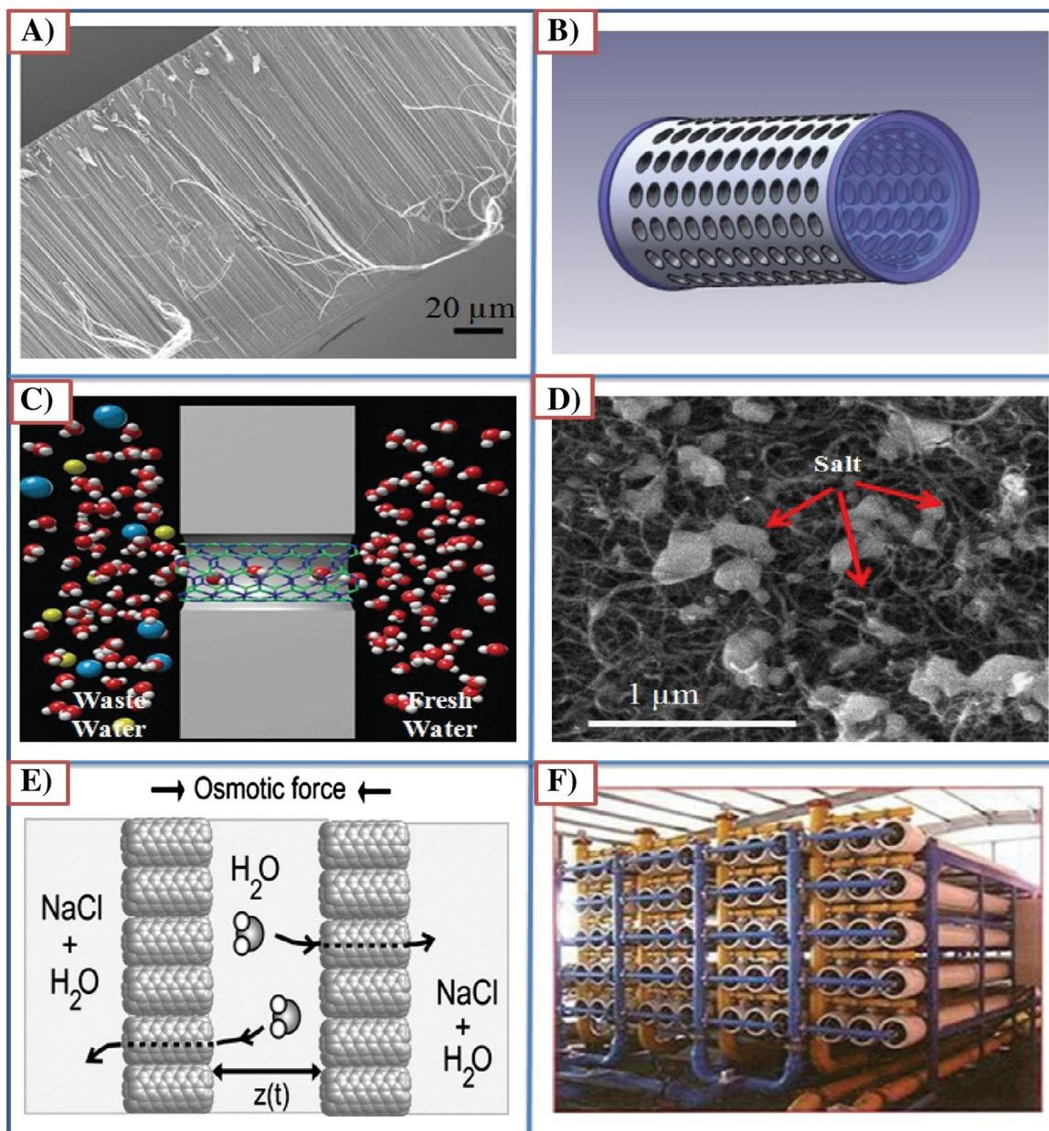
Fig. 5. Structures of some CNT membranes. Shown are (a) cross-sectional scanning electron microscope (SEM) image of a pristine CNT membrane; (b) CNT based water filter with cylindrical geometry; (c) movement of water molecules through a CNT channel; (d) SEM image of scattered NaCl nanocrystals on CNT membrane surface; (e) movement of pure water molecules through CNT-membrane in osmotically imbalanced compartments, and (f) engineered CNT membranes in industrial set up. Source, [28].
