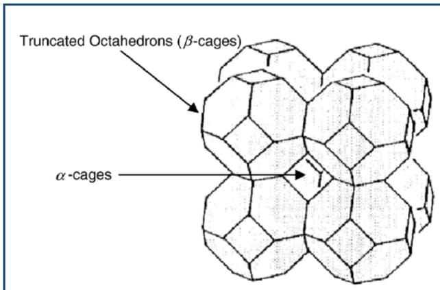
Fig. 2. Repeating unit of zeolite HS. Source, [23].
