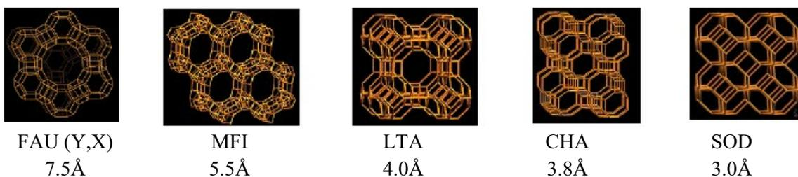
Fig. 3. Zeolite types. Source, [26].
