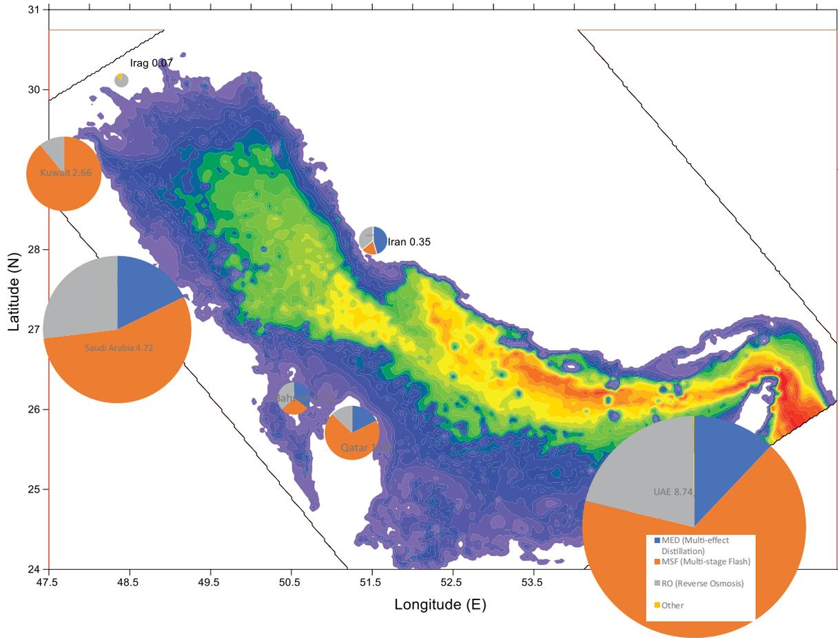
Fig. 2. Total desalination capacity by different desalination technologies in GCC countries.
