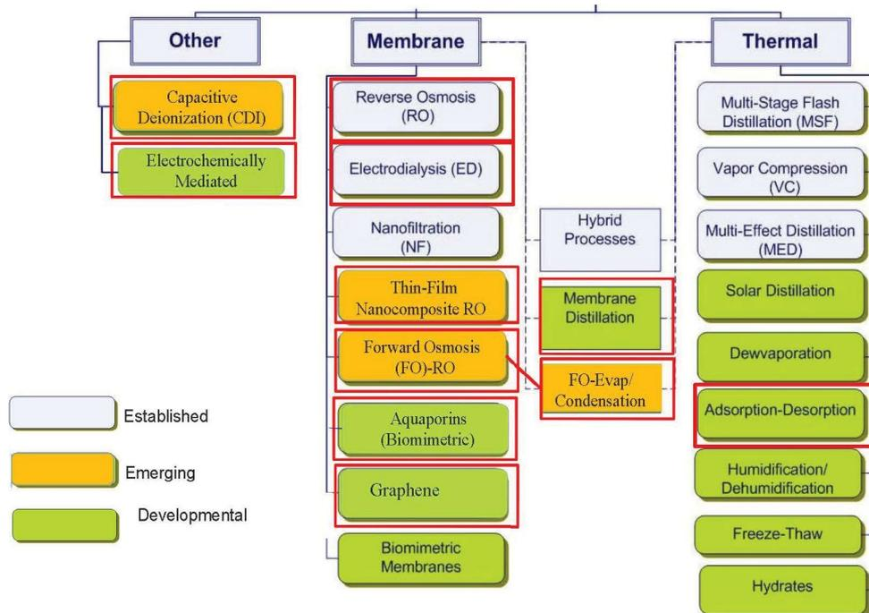
Fig. 8. Desalination technologies classification.
