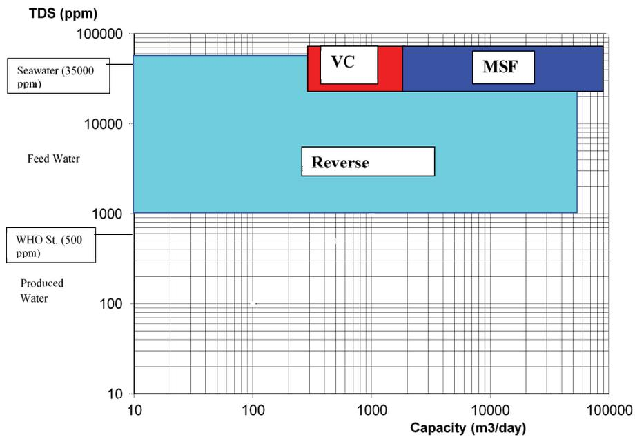
Fig. 5. Ranges of applicability for desalination technologies.
