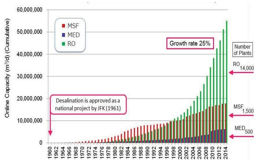
Fig. 6. Transition of the technology from distillation to membrane and expansion of the global desalination market.
