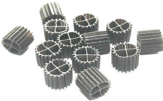
Fig. 2. Photographic view of bio carriers.
