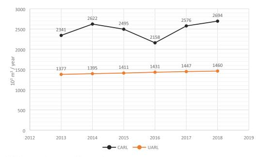
Fig. 3. Unavoidable losses in relation to total losses in the years 2013–2018 (company A).
