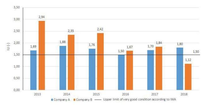
Fig. 5. Infrastructure leakage index - ILI.
