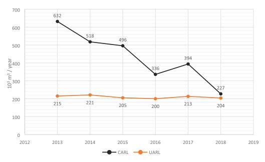
Fig. 4. Unavoidable losses in relation to total losses in the years 2013–2018 (system B).
