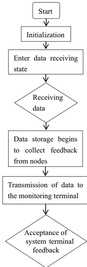
Fig. 3. Sink node workflow.
