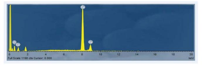
Fig. 5. EDX pattern of CuO nanoparticles.
