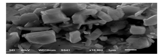
Fig. 4. SEM image of CuO nanoparticles.
