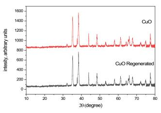
Fig. 15. X-ray diffraction spectra of CuO and CuO regenerated.
