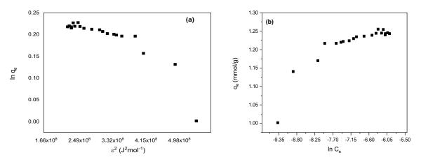
Fig. 10. Linearized isothermal sorption plots for AR57: (a) Dubbin-Radushkevich equation and (b) Temkin model.
