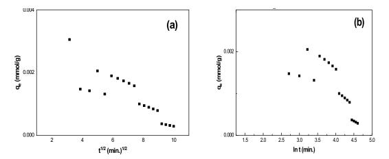
Fig. 12. Uptake kinetics modeling for AR57 with: (a) simplified model of resistance to intraparticle diffusion (Morris and Weber equation) and (b) Elovich equation.
