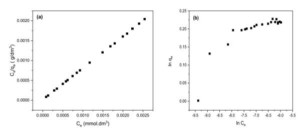
Fig. 9. Linearized isothermal sorption plots for AR57: (a) Langmuir equation and (b) Freundlich equation.
