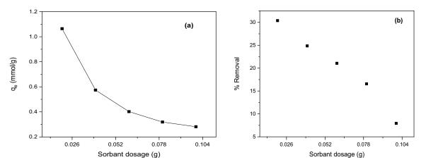
Fig. 8. Effect of sorbent dose (SD) on AR57 adsorption using CuO nanoparticles: (a) sorption capacity vs. SD and (b) % Removal vs. SD ( $C_0$ : 1.22 × 10<sup>-4</sup> M, *T*: 25°C, and pH 3).
