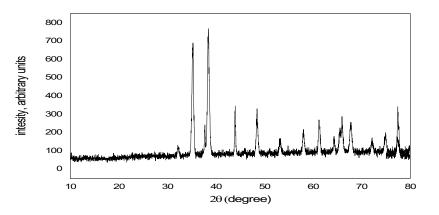
Fig. 2. X-ray diffraction spectra of CuO nanoparticles.
