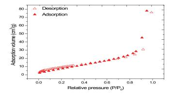
Fig. 3. N<sub>2</sub> sorption isotherm of CuO nanoparticles.
