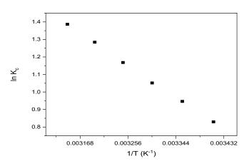
Fig. 13. Van't Hoff plots for AR57 adsorption onto the CuO nanoparticles adsorbent.
