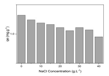
Fig. 14. Influence of NaCl on AR57 adsorption onto CuO nanoparticles ( $C_0$ : 1.2 × 10<sup>-4</sup> M, initial pH 3, *T*: 25°C, and sorbent dosage: 0.02 g, 25 mL).
