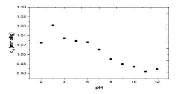
Fig. 7. pH effect on AR57 adsorption using CuO nanoparticles as adsorbent ( $T: 25^{\circ}C, C_0: 1.22 \times 10^{-4}M$ ).
