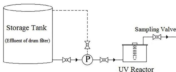
Fig. 1. Schematic of UV pilot.
