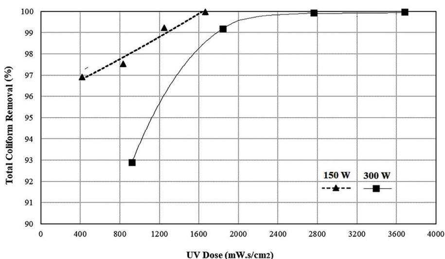
Fig. 8. Total coliform removal efficiency vs. UV dose.
