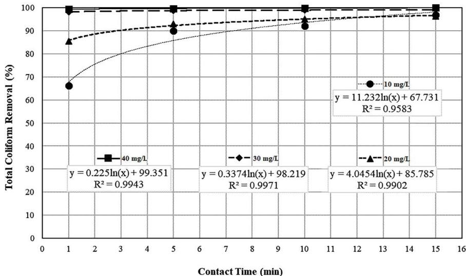
Fig. 10. Total coliform removal efficiency vs. ozone contact time for each ozone dose level.
