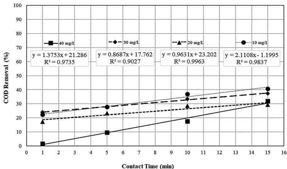
Fig. 6. COD removal efficiency vs. ozone contact time for each ozone dose level.
