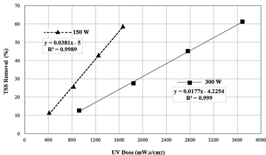
Fig. 3. TSS removal efficiency vs. UV dose.
