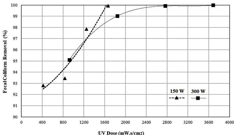
Fig. 7. Fecal coliform removal efficiency vs. UV dose.
