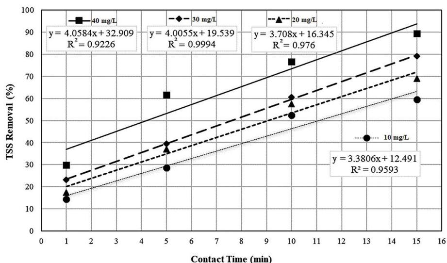
Fig. 4. TSS removal efficiency vs. ozone contact time for each ozone dose level.
