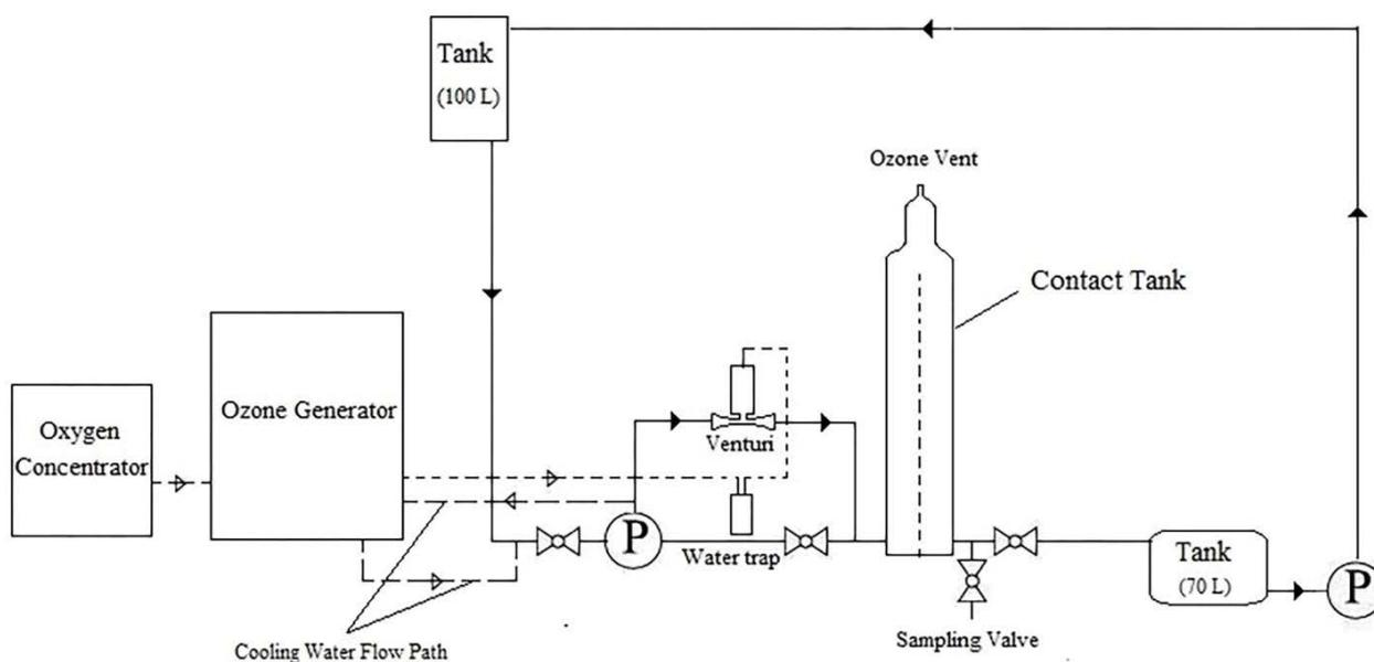
Fig. 2. Schematic of ozone pilot plant.
