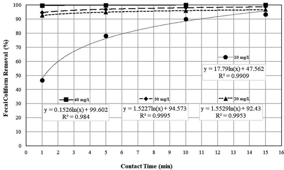
Fig. 9. Fecal coliform removal efficiency vs. ozone contact time for each ozone dose level.
