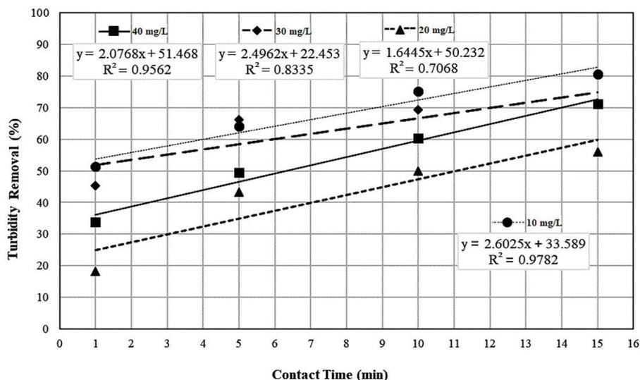
Fig. 5. Turbidity removal efficiency vs. ozone contact time for each ozone dose level.
