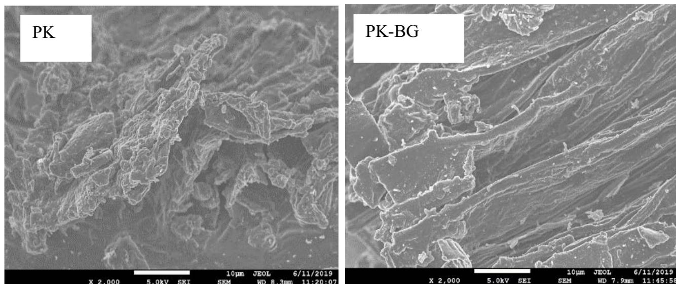
Fig. 2. SEM images of Pakis before and after adsorption of BG at 2,000 $\times$  magnification.
