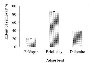
Fig. 2. Extent of removal of phosphate using various adsorbents (50.0 mL of 10.0 mg  $L^{-1}$  PO<sub>4</sub><sup>3-</sup> solution, 5.00 g of each adsorbent). Error bars at the top of the bar indicate standard deviation.
