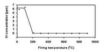
Fig. 4. Concentration of aluminum in the supernatant after interaction of brick clay fired at different temperatures with distilled water and (5.0 g brick clay, 50.0 mL distilled water, 10 min stirring, and 2.0 h settling).
