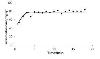
Fig. 7. Variation of the amount of phosphate adsorbed with contact time (50.0 mL of 10 mg  $L^{-1}$  phosphate solution, 5.0 g of BBC, 20 separate samples used for the analysis).
