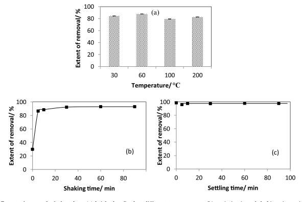
Fig. 3. Extent of removal of phosphate (a) brick clay fired at different temperatures, (b) optimization of shaking time with 1.0 h settling time, and (c) settling time at optimized shaking time (50.0 mL of 10.0 mg  $L^{-1} PO_4^{3-}$  solution, 5.00 g of each adsorbent). Error bars at the top of the bar indicate standard deviation in panel (a), and error bars were not indicated in panels (b and c) due to insignificant uncertainty.
