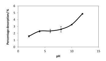
Fig. 9. Extent of desorption of phosphate pre-adsorbed on BBC for different initial solution pH.
