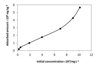
Fig. 6. Amount of phosphate adsorbed on BBC (50.0 mL solutions of different initial concentrations of phosphate shaken with 5.00 g of BBC, 30 min shaking, and 30 min settling time). Error bars are not indicated due to insignificant uncertainty.
