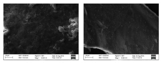
Fig. 5. SEM images for brick clay fired at 200°C before adsorption (left), and after adsorption of phosphate (right).
