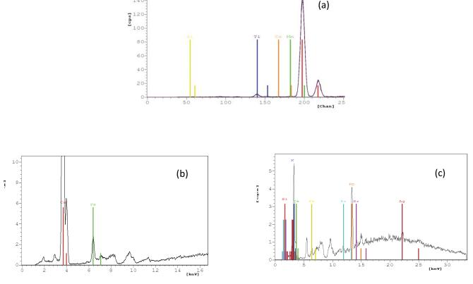
Fig. 1. XRF spectra of adsorbent samples: (a) brick clay, (b) dolomite, and (c) Feldspar. Lines indicate specific peak locations of respective elements.
