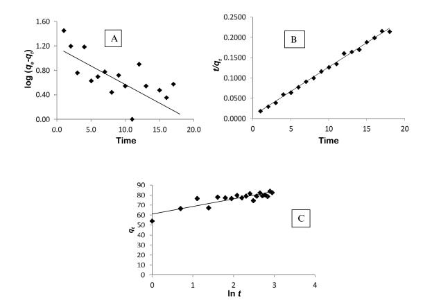
Fig. 8. Adsorption kinetics studies for removal of phosphate from brick clay: (a) pseudo-first-order kinetics, (b) pseudo-second-order kinetics, (c) Elovich model (50.0 mL of 10 mg L<sup>-1</sup> phosphate solution, 5.00 g of BBC) *t* is given in min and  $q_t$  is given in mg kg<sup>-1</sup>.
