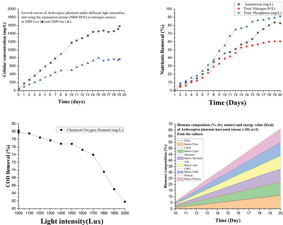
Fig. 5. *Arthrospira platensis* growth, nutrients removal, and biomass composition in the function of time and light intensity.
