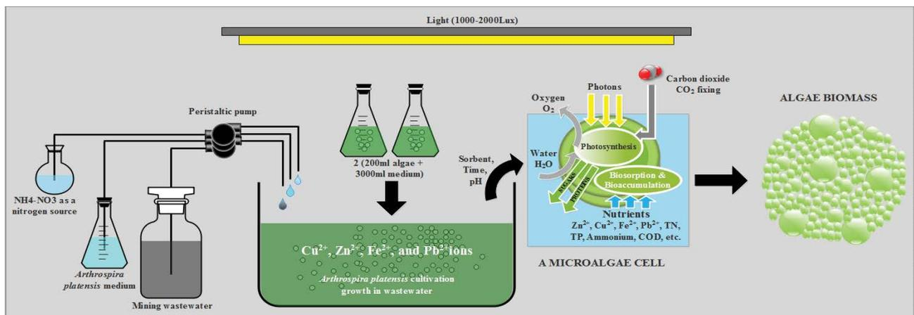
Fig. 4. Microalgae culture growth by biosorption and bioaccumulation for biomass production.
