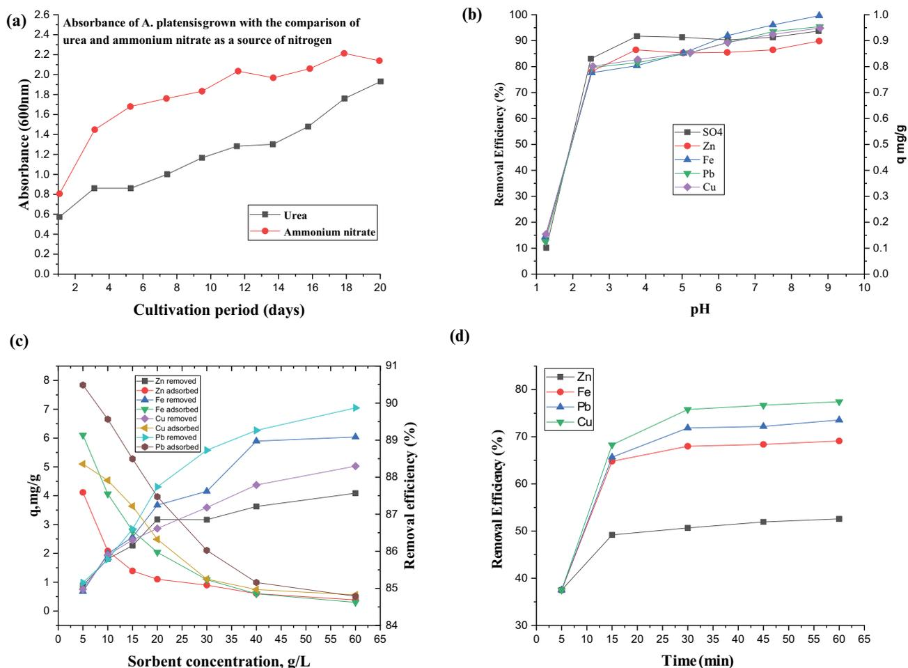
Fig. 6. The absorbance of *Arthrospira platensis*, the effect of pH, biosorbent concentration, and contact time on heavy metals biosorption from wastewater ( $T$  20°C;  $C_i$  45 mg L<sup>-1</sup>; pH 6.5; sorbent concentration 10 g L<sup>-1</sup>).
