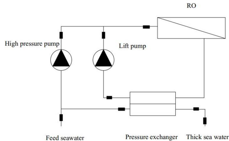
Fig. 4. Typical parallel reverse osmosis and functional exchange energy recovery process.
