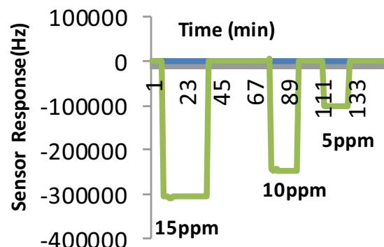
Fig. 3. QCM sensor responses of polyvinylpyrrolidone (MIPs + GO) towards 15, 10 and 5 ppm, respectively concentrations of methyl red.
