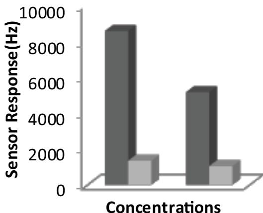
Fig. 2. Polyvinylpyrrolidone MIPs + GO sensor response towards 400 and 300 ppm, respectively concentrations of methyl red and methyl orange.
