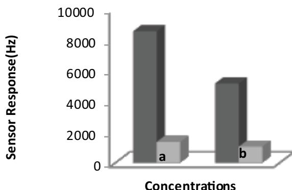
Fig. 1. Polystyrene (MIPs + GO) composite MIPs based sensor response towards 400 and 300 ppm, respectively concentrations of methyl orange and methyl red.
